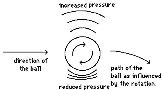
Figure 3. The influence of rotation on the flight of a ball. As the ball spins clockwise the air beneath the ball is accelerated thus reducing the pressure beneath the ball. The pressure above the ball is increased as the air is slowed, thus the ball moves from an area of high pressure to an area of low pressure.
