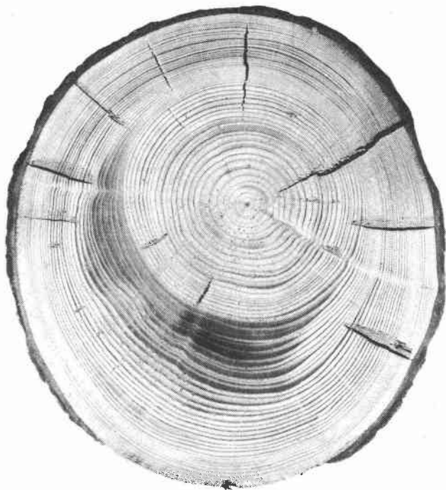
Cross section of log containing compression wood.
