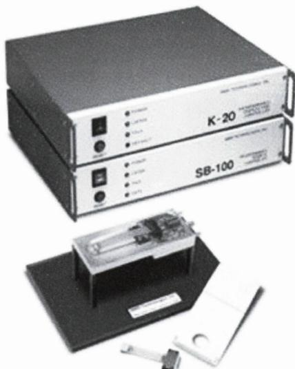
MMR's SB-100 Seebeck Measurement System allows users to make automatic measurements of the temperature-dependent Seebeck potential of metals, semiconductors and other electrically conductive samples over a temperature range from 70 K to 400 K, and from 200K to 730K. Sample mounting is simple permitting rapid interchange of samples. The Seebeck system is compatible with a variety of computers through an IEEE-488 (GPIA) or RS-232 interface. The MMR Programmable Seebeck Measurement System
