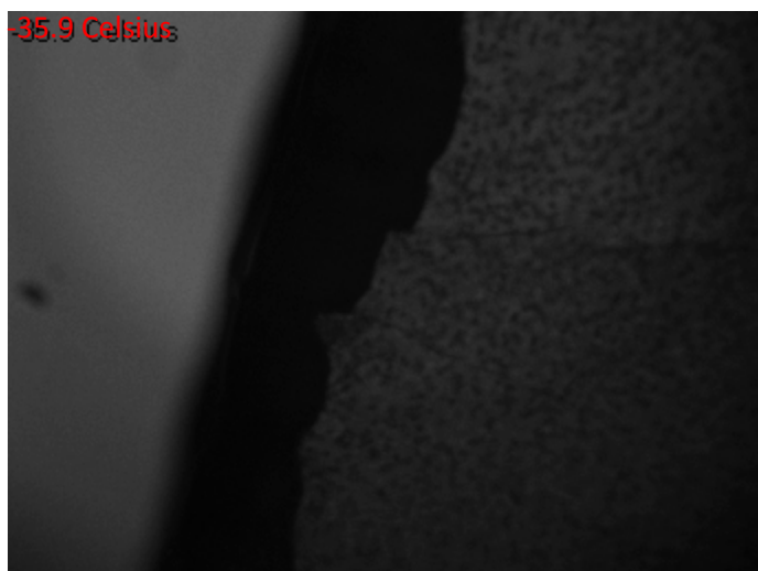
Figure 1- Stable primary drying of a sample of 20% hematocrit trehalose-loaded red blood cells. The dark section is the dried cake and the frozen sample is the lighter section with dots. The interface between the two is known as the drying front which travels radially in towards the center of the sample. This occurs at temperatures like the one overlaid in the upper left-hand corner which are below the cake collapse temperature, but not so low that the pressure cannot sublimate the ice crystals and dry the sample.
