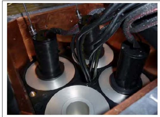
Fig. 2.6: One of the “quad” beta-gamma detectors and the partially assembled detector (Taken from (Cooper et al., 2011)).
