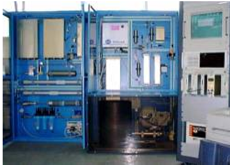
Fig. 2.2: A typical SPALAX detection system (Taken from (“CEA - Earth and Environmental Science,” 2013) ).
