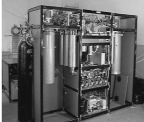
Fig. 2.12: General ARIX system (Taken from (Dubasov et al., 2005)).
