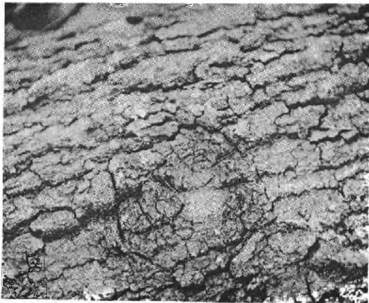
Bark distortion that clearly is an overgrown knot -- a defect in all diameter logs.
