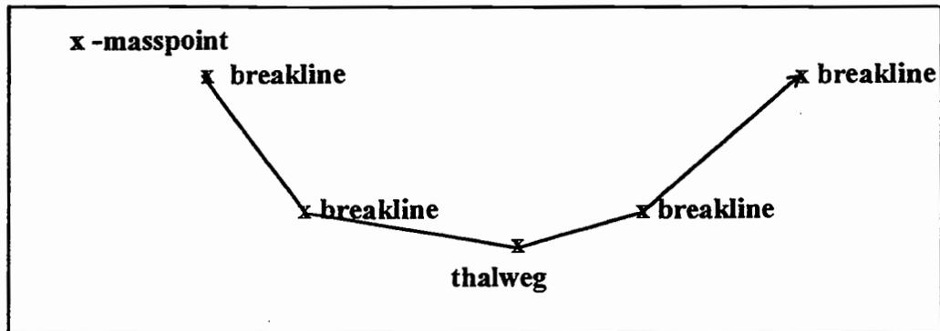
Figure 3. Example cross-section of stream channel surveyed for topographic maps including: thalweg points, breaklines and masspoints.
