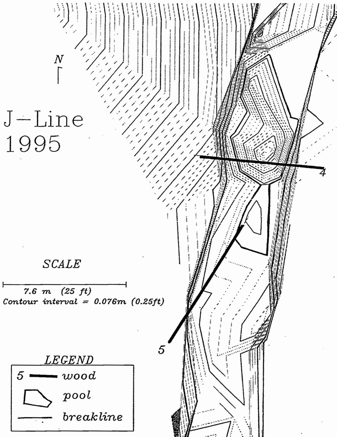
Figure 4. Topographic map of J-Line Creek in 1995, including tagged wood numbers four and five, top of bank and bankfull breaklines, and a residual pool.
