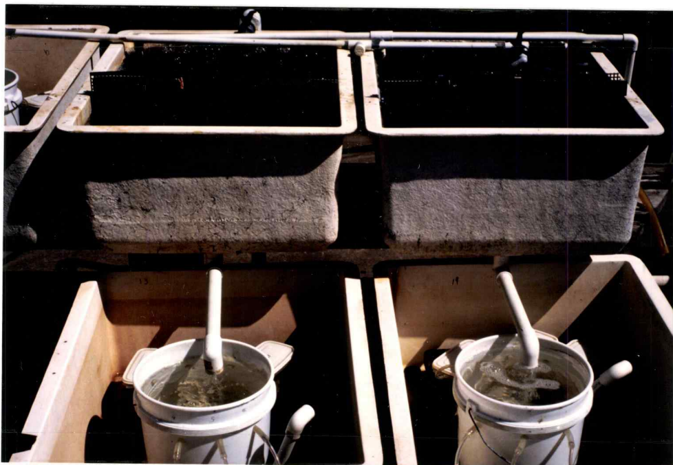
FIGURE 7.- Experimental apparatus, Summer Experiments. Upper tanks: salmon effluent (left) and ambient seawater (right) stocked with 18 g/l Palmaria mollis . Lower tanks hold the water reservoirs and the experimental units.
