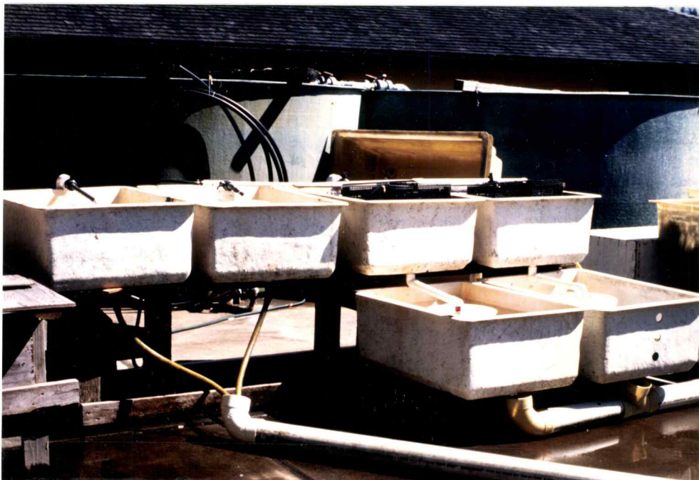
FIGURE 6.- Experimental apparatus, Summer Experiments. Initial stocking density of bivalves was 5 g per replicate ( n=3 ) during Summer Experiment #1 (June 3 - July 4, 1991) and 3 g in Summer Experiment #2 (July 19 - Aug 17, 1991).
