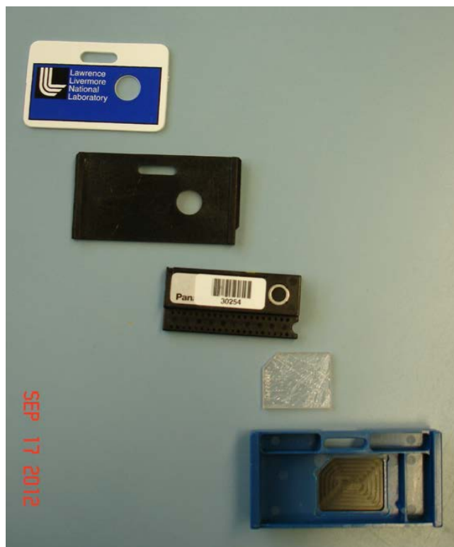
Figure 1. LLNL Dosimeter Case with Panasonic UD-810 and CR-39 Foil
