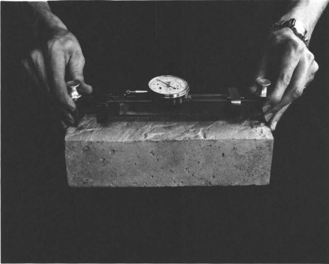
Figure 23. Measurement of Shrinkage
