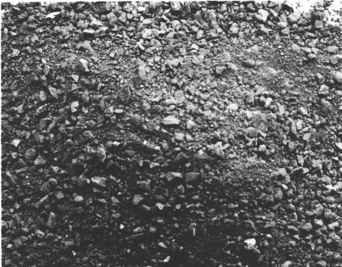
Figure 11. Fine Expanded-Shale No. 2
