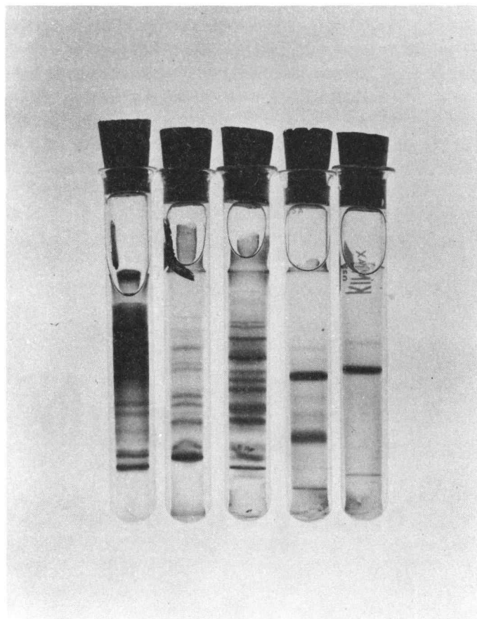
Figure 9. Disc-gel Electrophoresis of Halophilic Alkaline Phosphatase Preparations. From left to right: crude extract, 40-55% acetone fraction, 60-80% ammonium sulfate fraction, enzyme fraction from Column II, and enzyme fraction from Column III.
