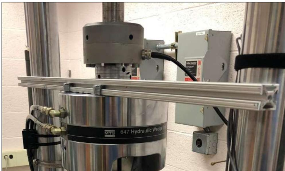
Figure 8: Anti-Spin Fixture for Upper Hydraulic Wedge Grip [38].
