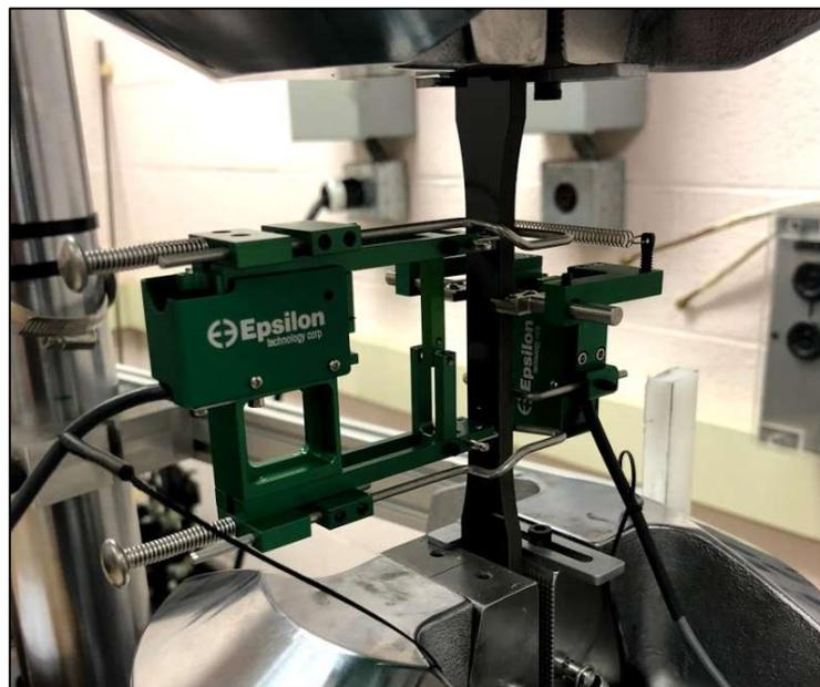
Figure 4: Axial (left) and Transverse (right) Extensometers during a Tensile Test
