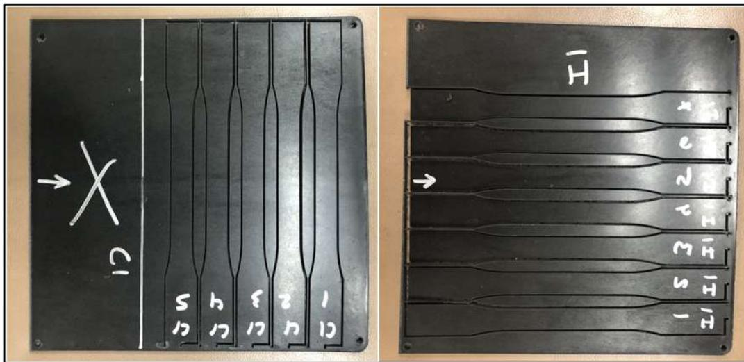
Figure 13: Cross-Flow (left) and In-Flow (right) 40% GF-PP Coupons [38].
