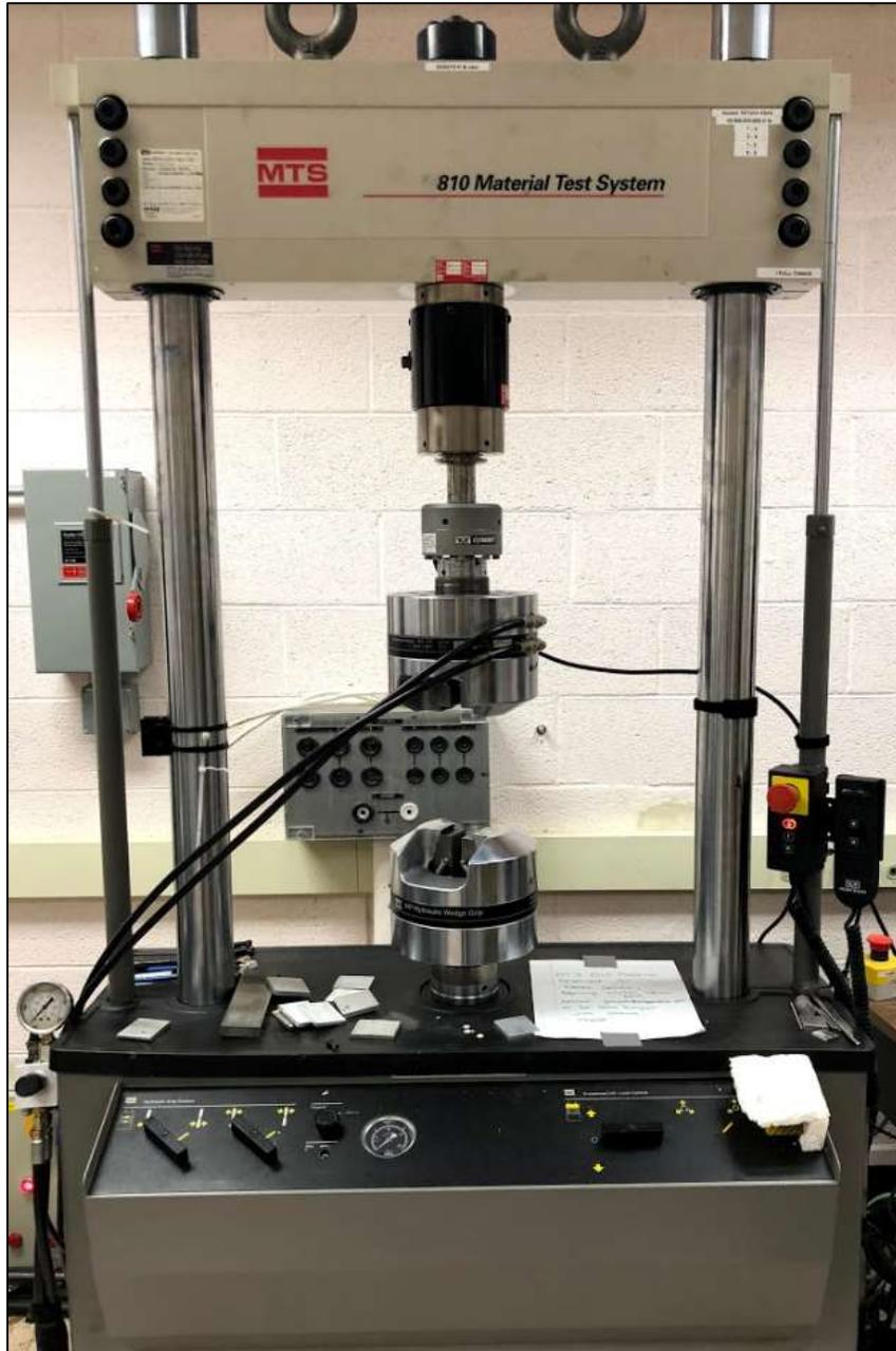
Figure 1: MTS 810 Hydraulic Load Frame at OSU
