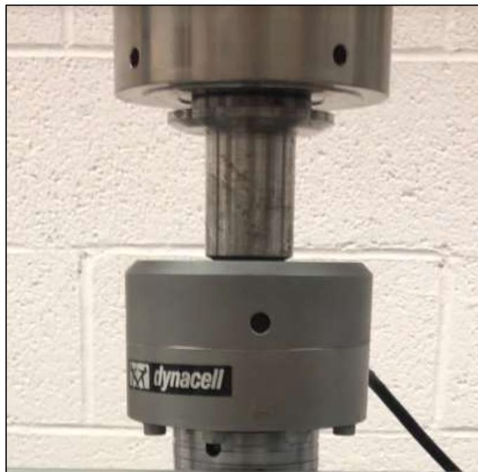
Figure 3: Instron "dynacell" +/-25kN Dynamic Load Cell
