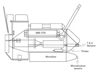
FIG. 3. Schematic of SeaSoar as equipped for use during the COAST experiment.
