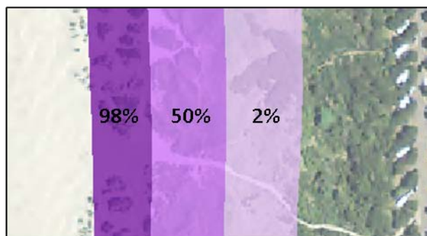
Figure 18. Conceptual diagram illustrating the delineation of the coastal change hazard zones, which are defined probabilistically based on the 95% confidence interval (CI) for the cross-shore distribution of expected erosion distances.
