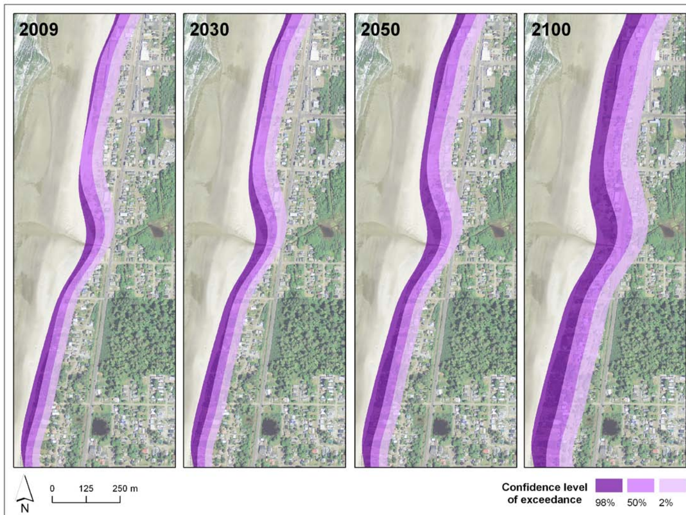
Figure 19. Coastal change hazard zones associated with the 1% annual chance TWL event for a section of the Rockaway littoral cell for 2009, 2030, 2050, and 2100.
