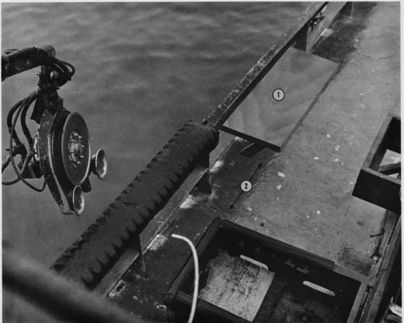
Figure 6. Block rigged for long lining. A folding platform is anchored to the rail as a ready base for pots.
