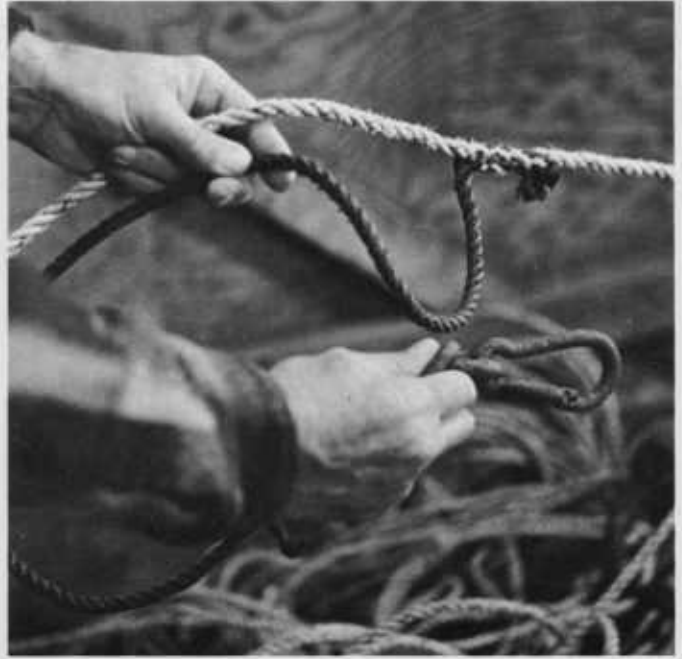
Figure 5C. Rigging details of gangeon. Gangeon should be two feet in length with one end spliced into the ground line and the other spliced into a 3-inch spring-loaded snap.
