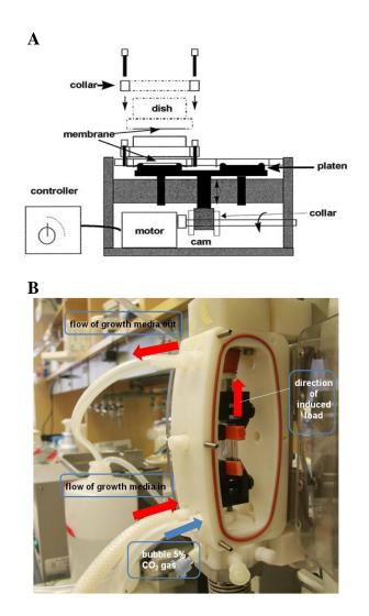
**Figure 2.** (A) Diagram of biaxial loading device similar to loading device used in this experiment [27], (B) View of BioDynamic test device used for uniaxial loading. Cell culture medium is flowed through test device with a 5%  $CO_2$  bubbler to pH balance growth media.
