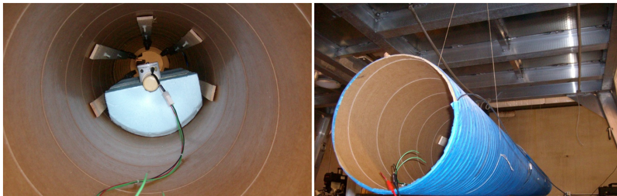
Figure 5 - Magnetic sensor undergoing magnetic calibration
