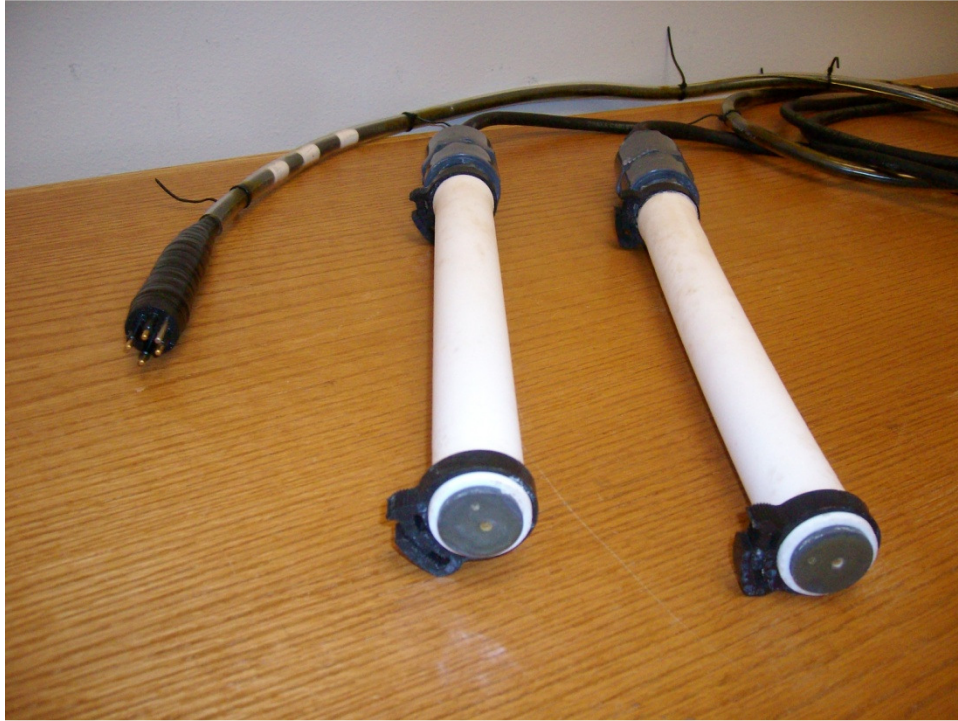
Figure 3 - Electric field probes and wet-mate interconnect cable
