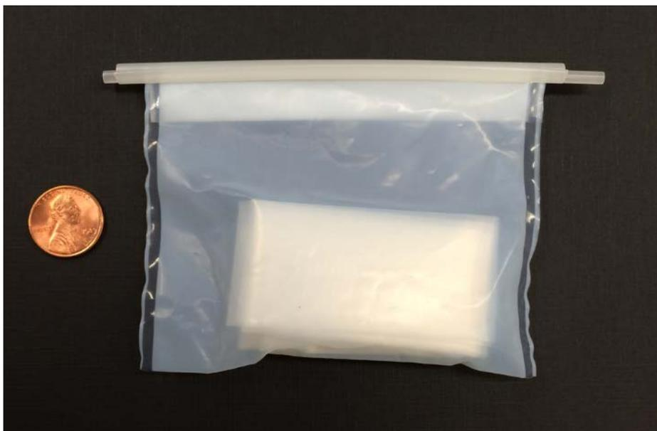
Figure 2.1. LDPE passive sampling strip in PTFE bag.
