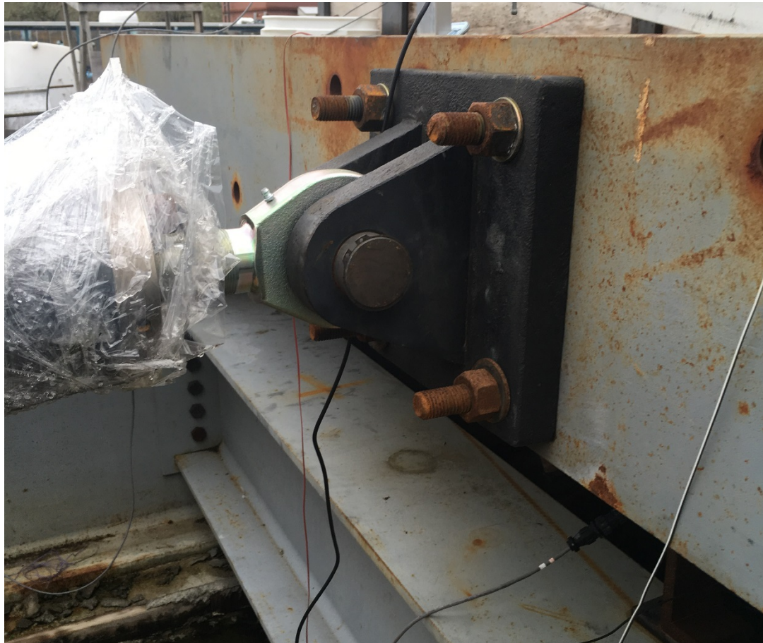
Figure A 11: Bolted Connection between Actuator Piston and Shake Table Cross-Beam
