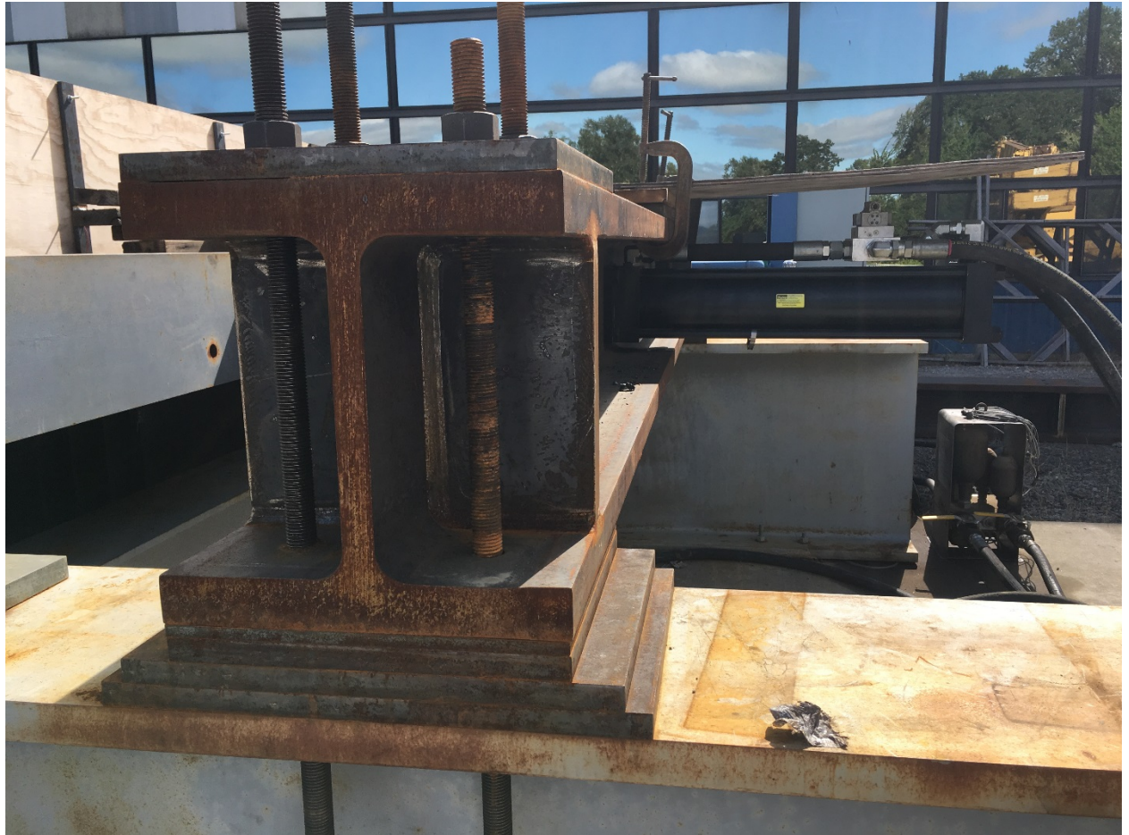
Figure A 10: Actuator Beam Set-up and Connection
