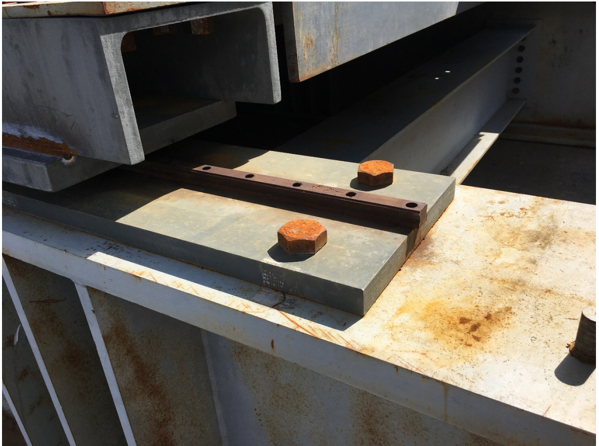
Figure A 3: Linear Motion Rail on Top of and in Parallel with W40x324 Shake Table Framing Beam.
