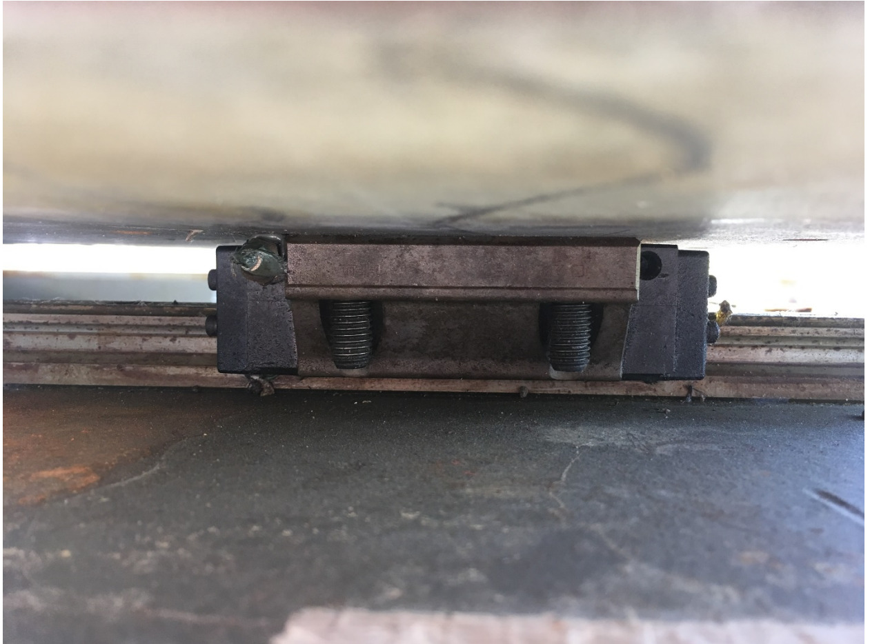
Figure A 5: Linear Motion Bearing Mounted on Linear Motion Rail
