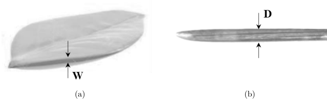
Fig. A.1 The thickness ( W ) and diameter ( D ) of leaf (a) and needle (b) to define ignition sensitivity index (ISI).
