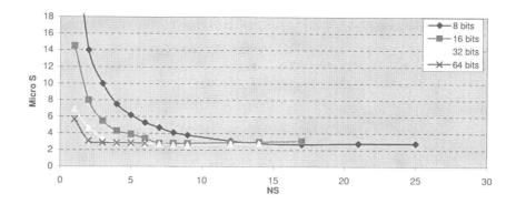
FIGURE 5.4: Total computational time for radix-8 kernel, 256 operands.
