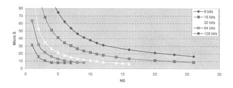
FIGURE 5.2: Total computational time for radix-4 kernel, 1024 operands.
