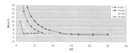
FIGURE 5.3: Total computational time for radix-2 kernel, 256 operands.
