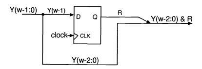
FIGURE 3.5: Word-serial bit shifter.
