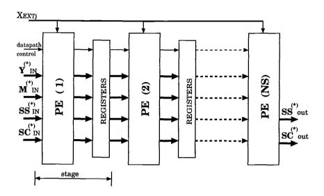
FIGURE 3.2: Top Level Diagram of Kernel datapath.
