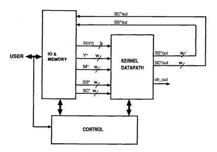
FIGURE 3.1: System Level Diagram of Modular Multiplier.
