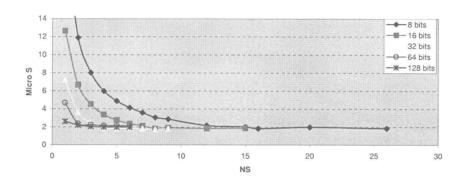
FIGURE 5.1: Total computational time for radix-4 kernel, 256 operands.
