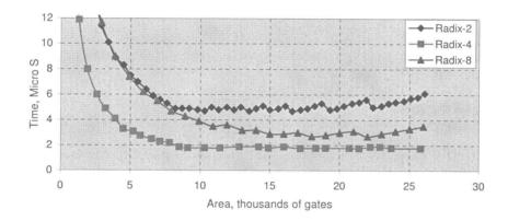
FIGURE 6.1: Total computational time compared to area usage, for 256-bit operands.
