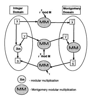
FIGURE 1.1: Modular multiplication using MM.
