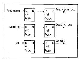
FIGURE 4.3: Control signals' propagation between two pipeline stages.
