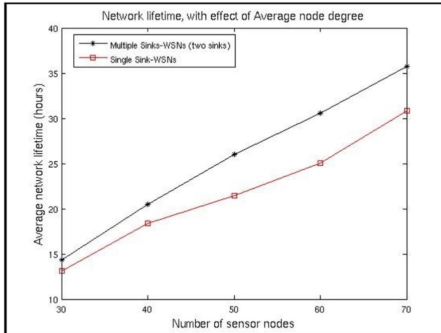
Figure 5.6: Network Lifetime, with effect of average node degree: Network load = 30 source nodes, Transmission range = 35.
