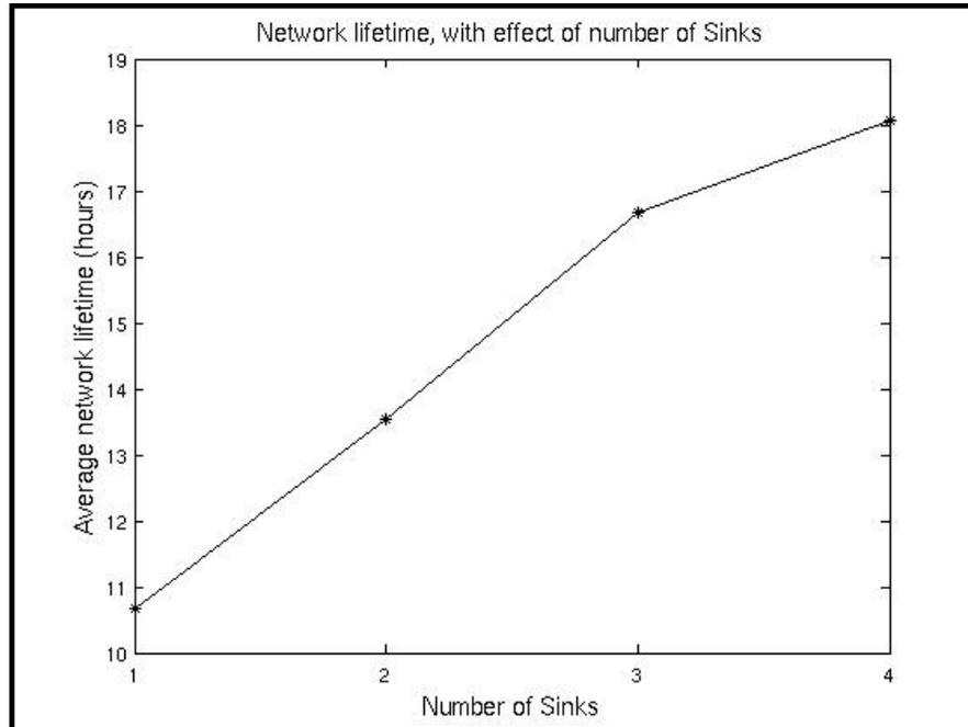
Figure 5.5: Network Lifetime, with effect of number of sinks: Number of sensor nodes =40, Network load = 40 source nodes, Transmission range = 35.
