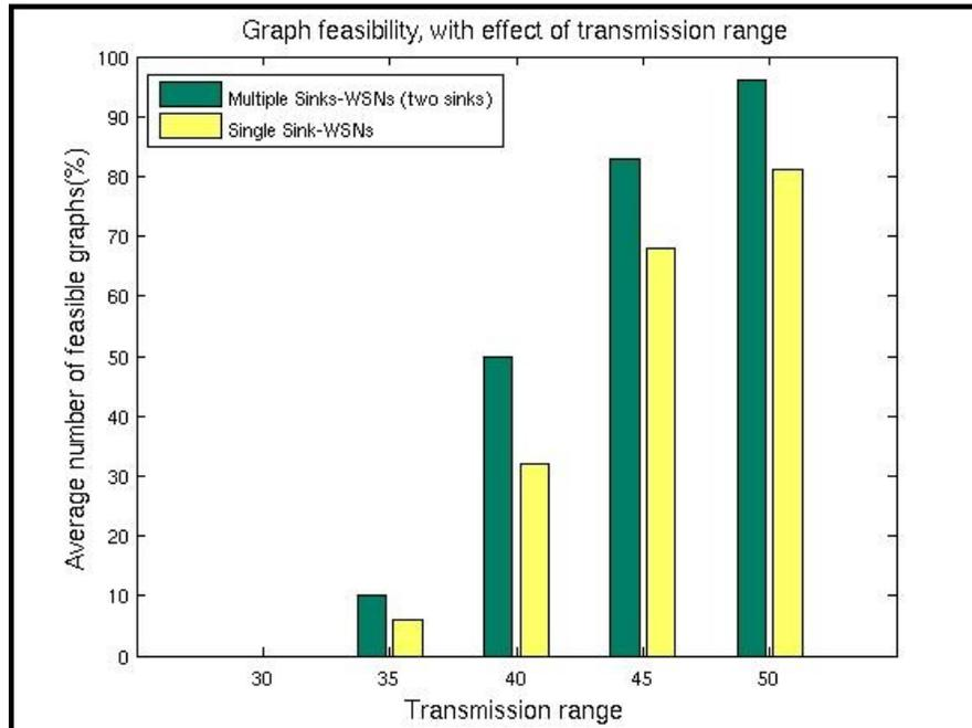
Figure 5.4: Graph feasibility, with effect of transmission range: Number of nodes = 40, Network load = 40 source nodes.
