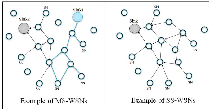
Figure 1.2: Sample WSN with multiple sinks (two sinks) versus WSN with single sink node
