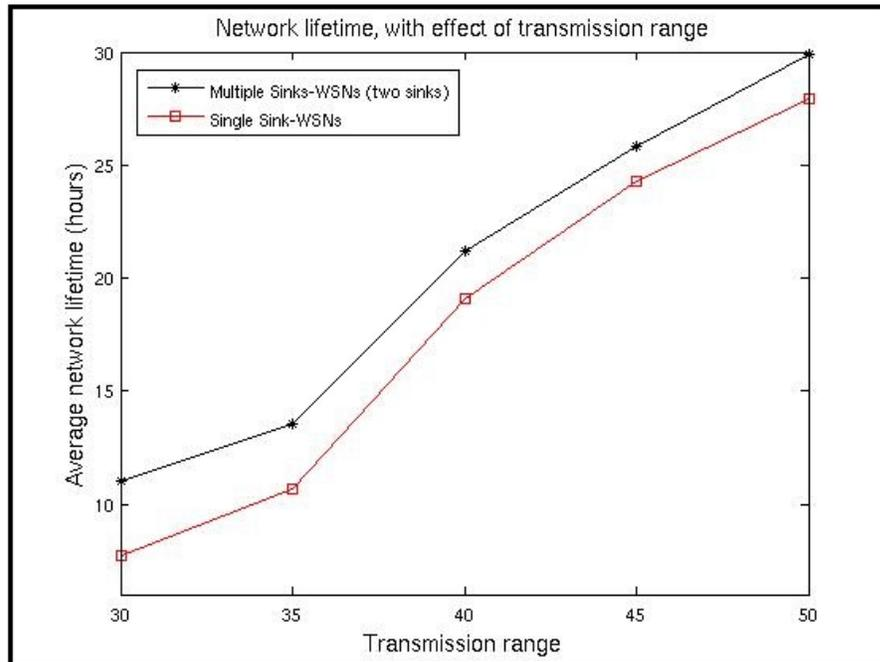
Figure 5.8: Network Lifetime, with effect of transmission range: Number of nodes = 40, Network load = 40 source nodes.
