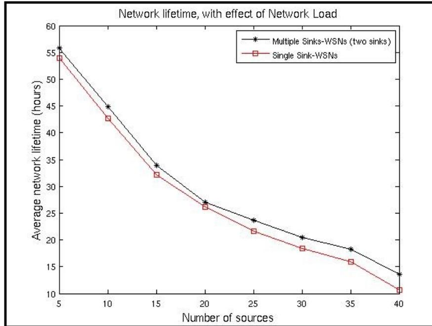
Figure 5.7: Network Lifetime, with effect of Network Load: Number of sensor nodes = 40, Transmission range = 35.
