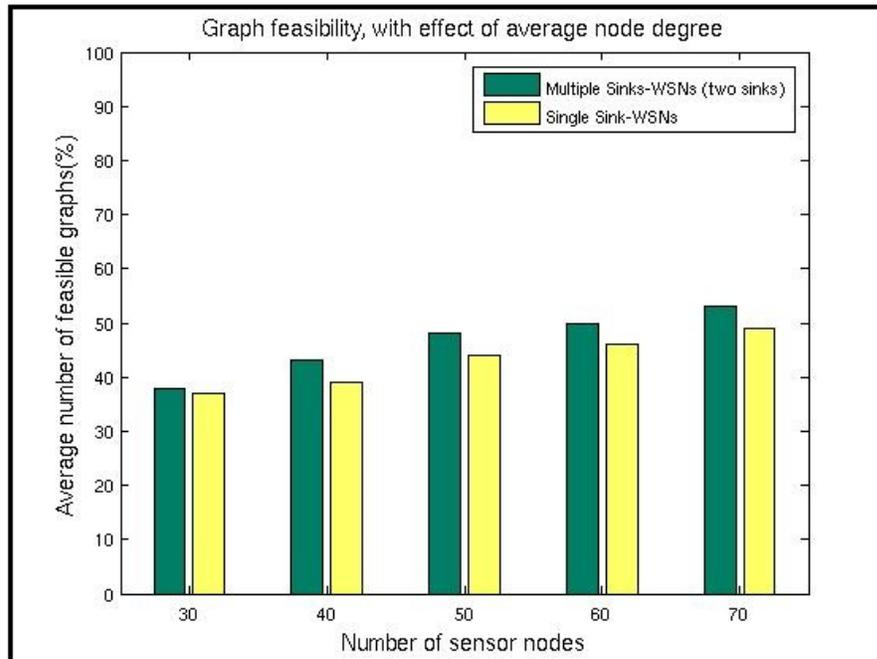
Figure 5.2: Graph feasibility, with effect of average node degree: Network load = 30 source nodes, Transmission range = 35.
