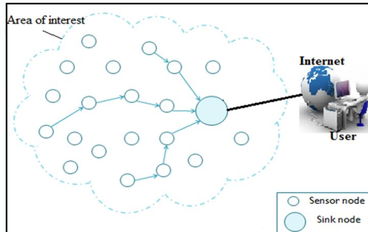
Figure 1.1: Sample Wireless Sensor Network (WSN).
