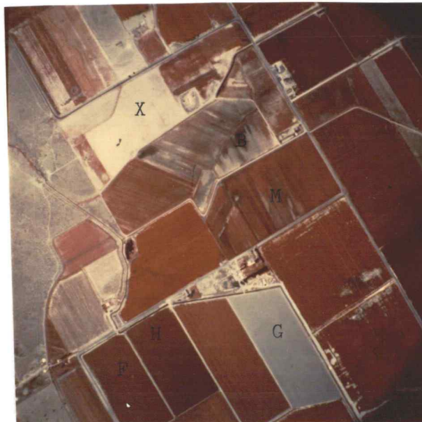
Figure 68. A mid summer scene - July 9, 1979. Most patterns are subdued by vegetation, especially in fields F and H. Damaged crops (blue) near supply ditch in F indicates furrow or border strip. H has hand move system which is hard to tell unless viewed very closely. Straight wetting strips can be seen, length of strips indicates that it is hand move system. Furrow irrigated fields at M shows effects of uneven water distribution, crops in the lower middle part of the field are poorly developed. B is a harvested bluegrass field that is being irrigated by furrow irrigation. Also see fallow land at X. The dark blue field at G is a clipped garlic field, which looks like a dry field. Approximate image scale is 1:23,000.
