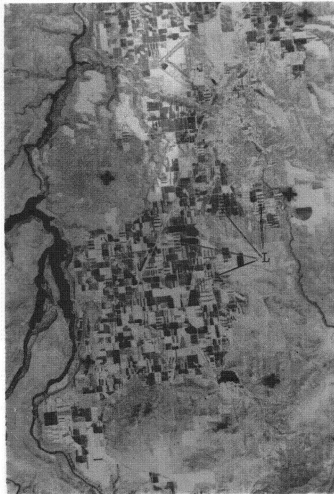
Figure 62. Landsat RBV image for southern part of North Unit Deschutes Irrigation District for June 8, 1978. Thin, dark gray strips marked by letter L show the wet strips of sprinkler systems. Reproduction resulted in reduction of the scale. Image scale is approximately 1:230,000.
