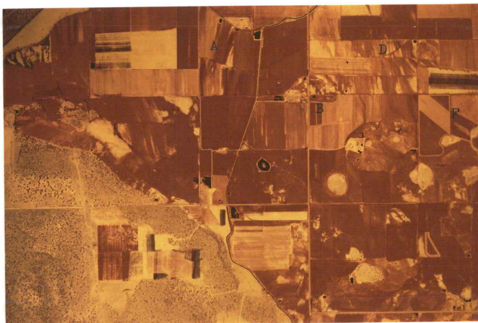
Figure 71. Wild flooding of fields at A and D using basin irrigation. Controlled flooding by furrows at F and by border strip at B can also be seen. Approximate image scale is 1:26,000.
