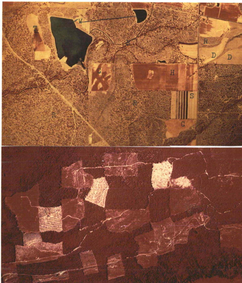
Figure 67. Different land uses: the image on the top shows reservoirs, range, and agricultural fields. Letters stand for types - water (W), range (R), side-roll (S), hand move (H), terrace (T), contour ditch (C), dry farming (D). The lower image shows forests and various age clearcuts. Compare the texture - smooth for water, coarse for forests, and fine for crops. Approximate scale is 1:26,000.
