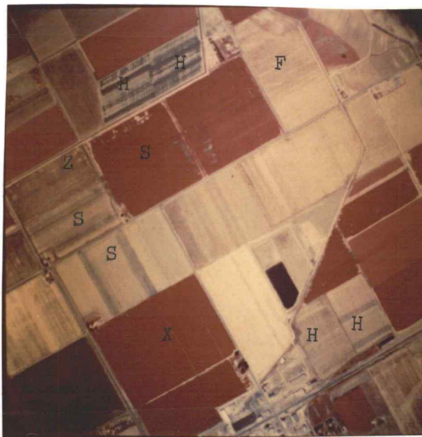
Figure 69. A late summer scene - August 5, 1979. Harvested fields (whitish) show many details. Wetting patterns of overlapping sprinklers are seen both in S (side-roll) and H (hand move) systems. Furrow lineations can be seen at F. Side-roll laterals can be seen at X shown by thin white lines. Also notice the mottling in field Z as a result of uneven water retention. Approximate scale of the image is 1:23,000.
