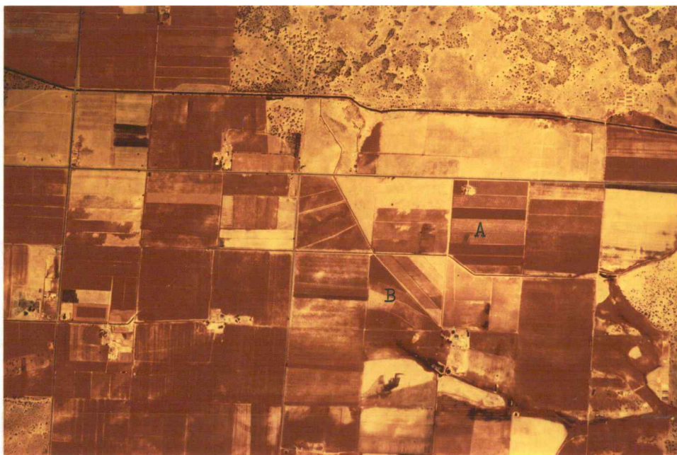
Figure 72. Corrugations are shown on level land and on rough surface at A and B respectively. Approximate image scale is 1:26,000.
