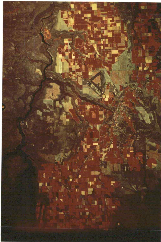
Figure 64. U-2 CIR photograph for central part of North Unit Deschutes Irrigation District for August 2, 1978. Reproduction resulted in reduction of the scale. Approximate image scale is 1:268,000.
