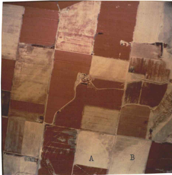
Figure 70. A late summer scene - August 5, 1979. Center pivot system with irrigated corners using different methods. There are two center pivot systems at A and B. The corner of A is irrigated by guns. The wetting pattern of individual guns without a strip is seen in the harvested corner. The corner of B is irrigated by hand move as can be seen in the wetting strip with faint sprinkler patterns. Approximate image scale is 1:23,000.
