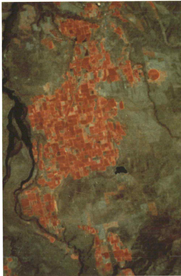
Figure 61. Landsat MSS color composite print for southern part of North Unit Deschutes Irrigation District for June 22, 1979. Reproduction resulted in enlargement of scale. Approximate image scale is 1:210,000.
