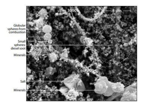
Figure 1. Electron micrograph of PM sampled on a filter near a street; diesel soot (small grey spheres)<sup>3</sup>.
