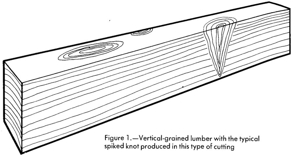
Figure 1.—Vertical-grained lumber with the typical spiked knot produced in this type of cutting
