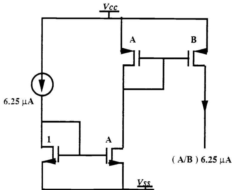
Fig. 4.5. Current Carrying Before Mirroring.
