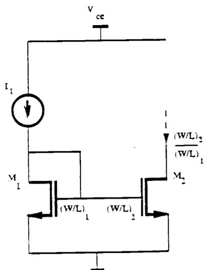
Fig. 2.4. Simple Current Mirror.
