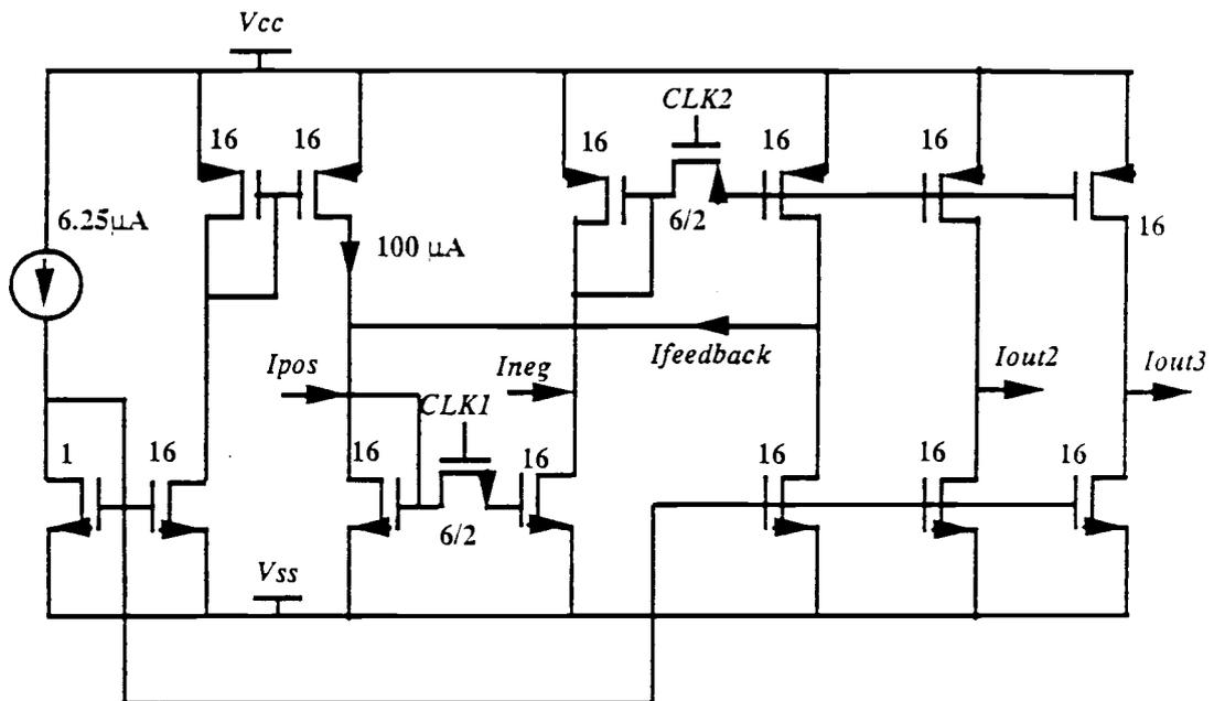
Fig. 4.4. SI Integrator with differential inputs and two outputs.
