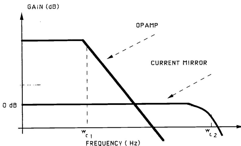
Fig. 2.2. Comparison of Frequency Responses of a Simple Current Mirror and an Opamp.
