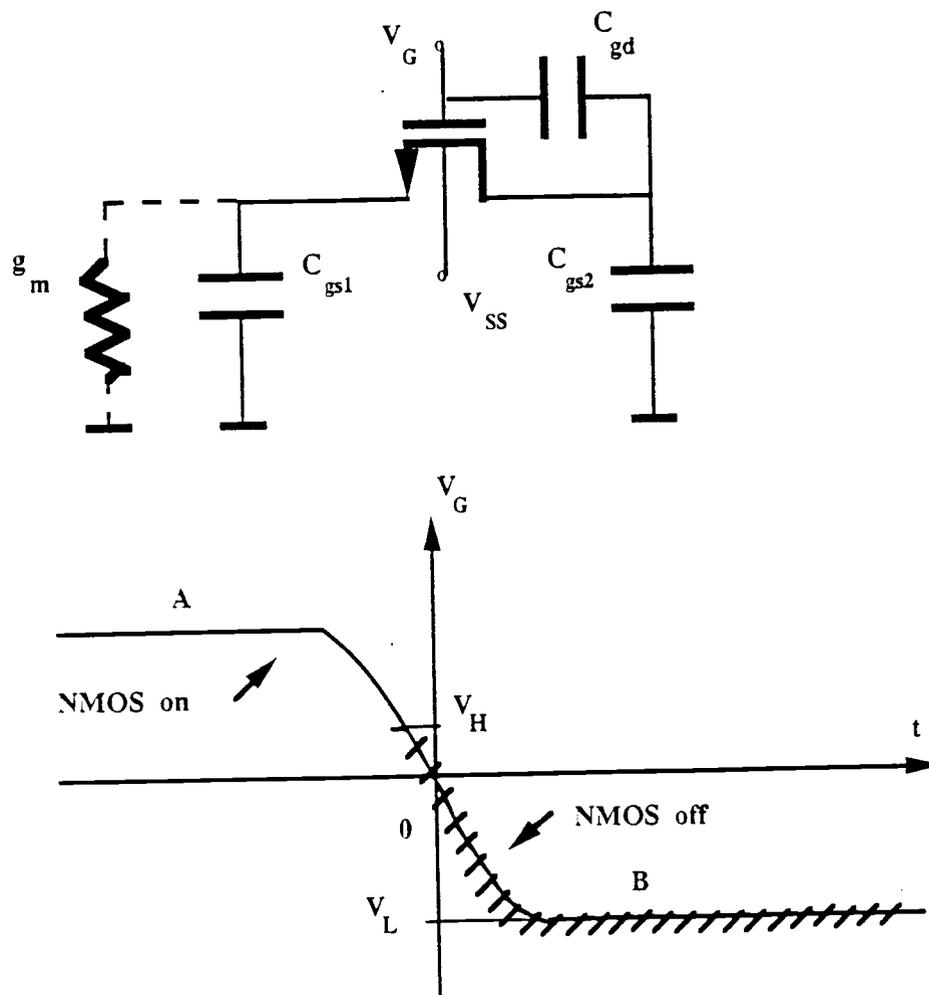
Fig. 2.14. Clock Feedthrough.
