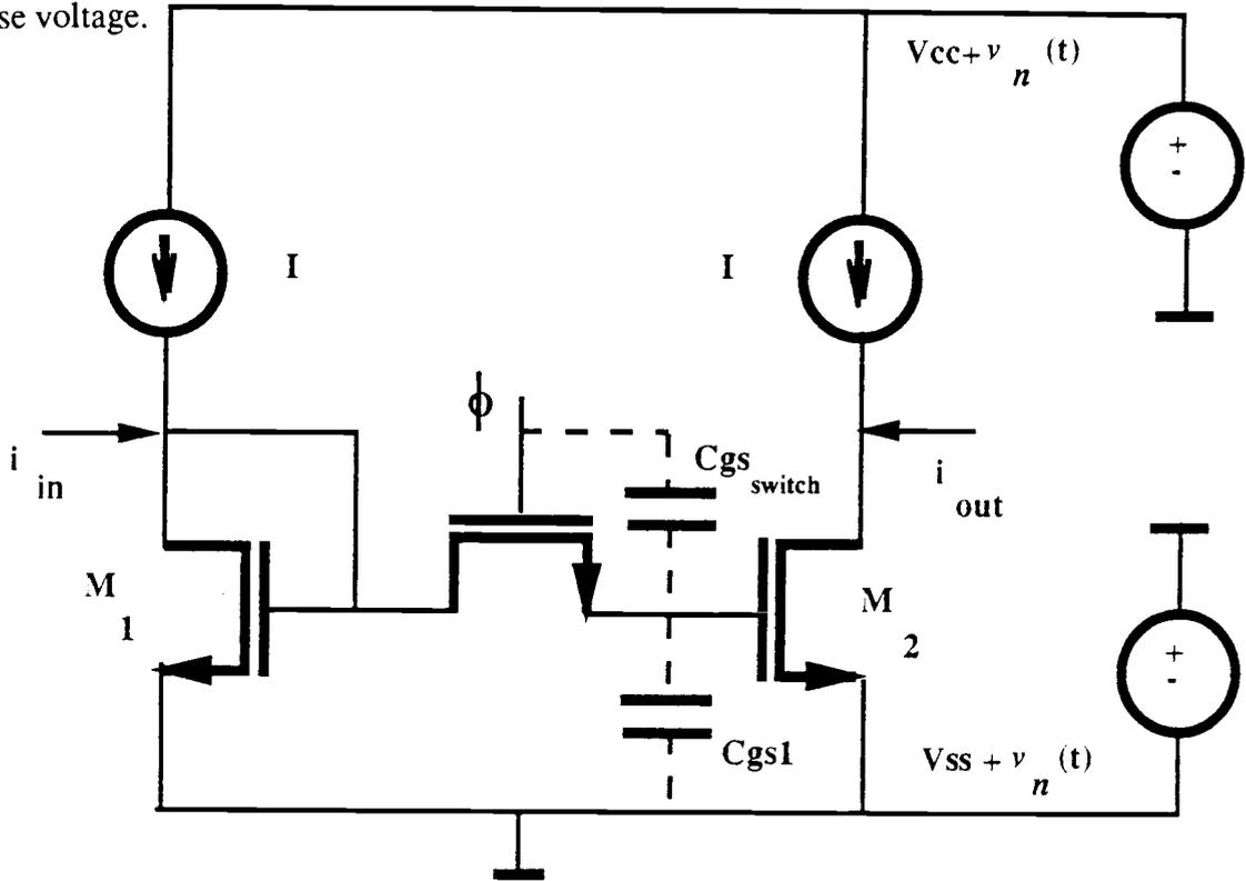
Fig. 2.3. Simple Current Mirror with the Noisy Power Supplies.
