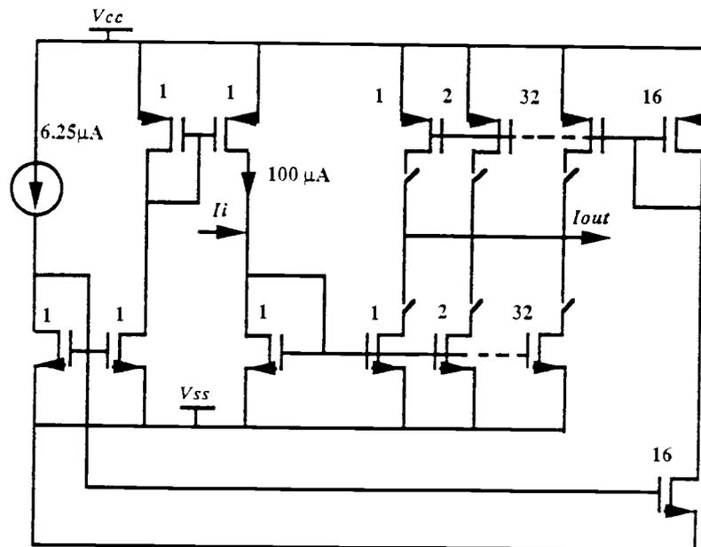
Fig. 4.1. Input Gain Programming Block.
