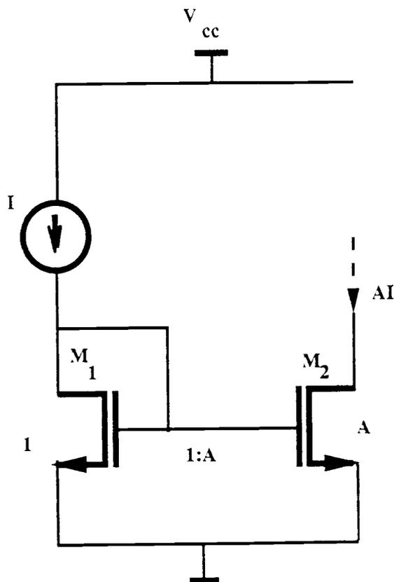
Fig. 2.6. Scaling in a Simple Current Mirror.
