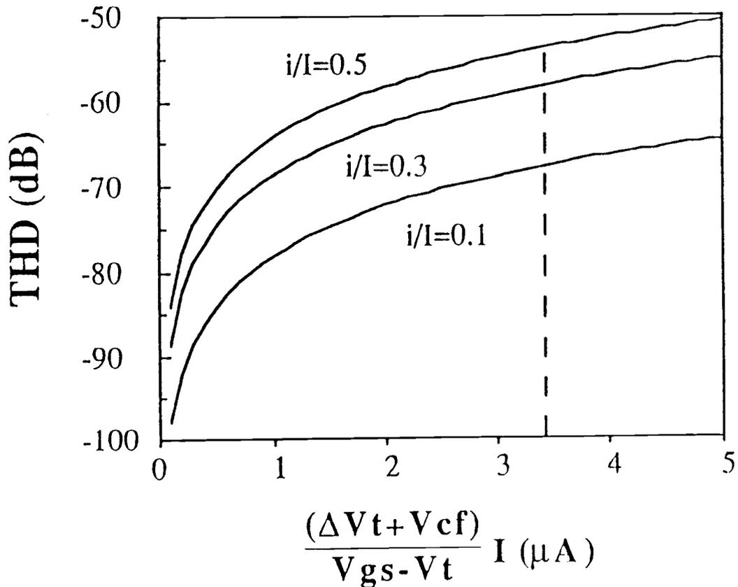
Fig. 2.19. Total harmonic distortion due to the clock-feedthrough and mismatches.
