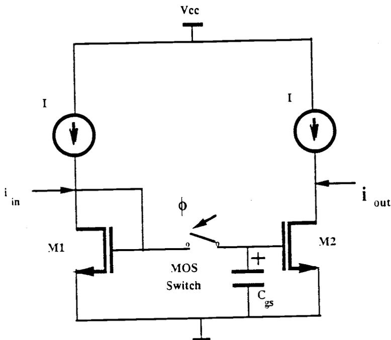
Fig. 2.9. Holding mode in an SI Integrator.
