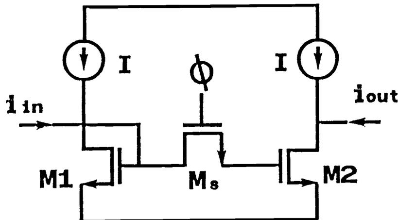
Fig. 2.18. Clock Feedthrough in a Track-and-Hold Circuit.
