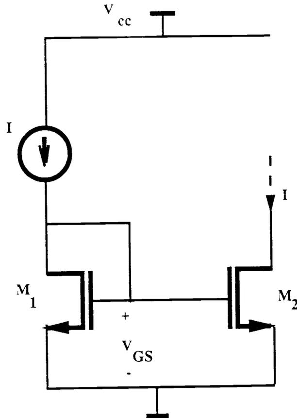
Fig. 2.1. Basic Current Mirror Structure in SI Circuits.
