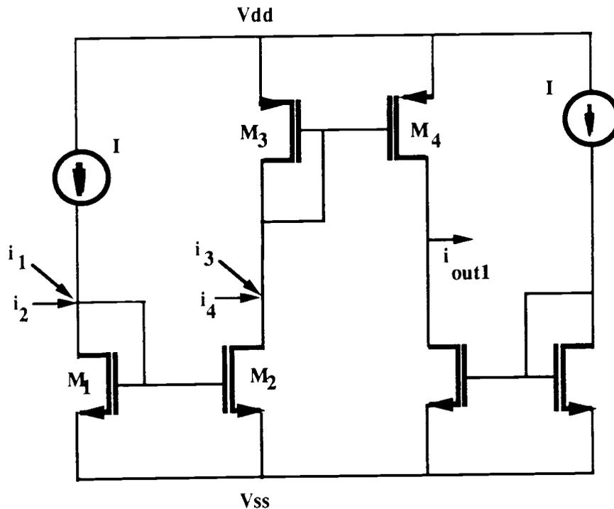
Fig. 2.5. Current Amplifier for Inversion, Summation and Subtraction in SI Circuits.
