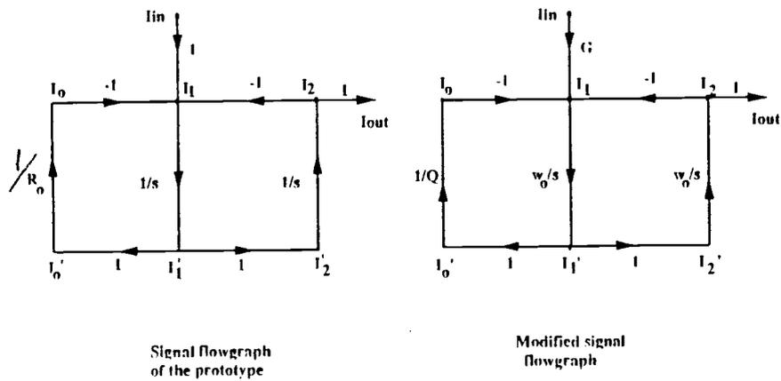
Fig. 3.2. Signal Flowgraphs of the Prototype Before and After Modification.
