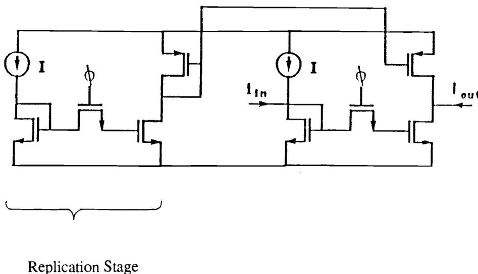
Fig. 2.17.a. Clock Feedthrough Cancellation Technique with the Proposed Circuit.
