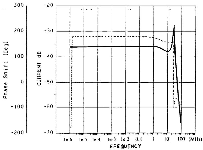
Fig. 4.7. Simulations of Frequency Responses of a Current Amplifier with the Source Follower.
