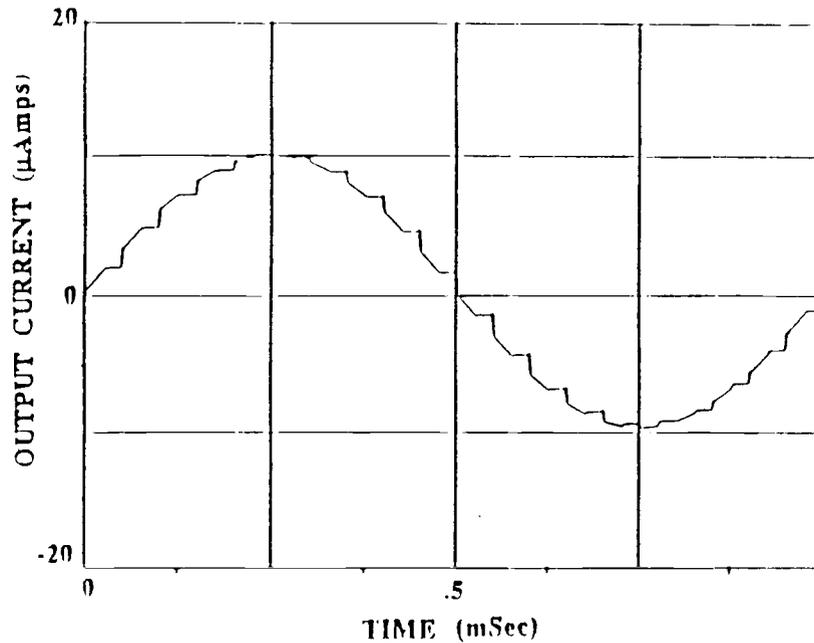
Fig. 2.17.b. SPICE Results of the Proposed Circuit.
