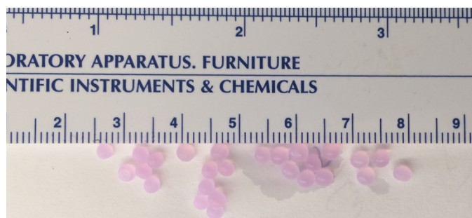
Figure 20: Size of biotic beads shown against a VWR ruler for scale. Beads were 2-3 mm in diameter. Pink color is a result from resazurin indicator reacting with oxygen in the surrounding environment.
