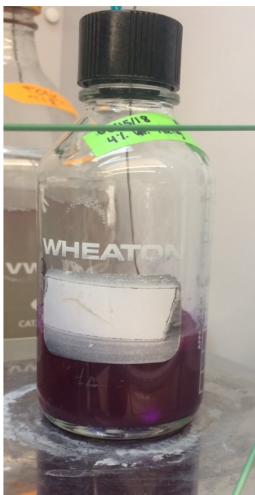
Figure 6: 4% wt sodium alginate gel transitioning from blue to pink to grey. Bottle capped with screw cap and rubber septum.
