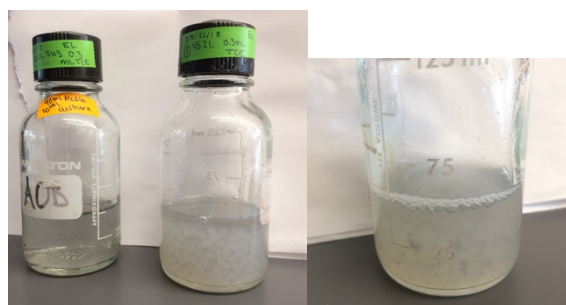
Figure 16: Photo of suspended and encapsulated cells for set 1 on the 3 rd day of the experiment (left). Photo of the encapsulated cells 9 days after start of experiment (right). Media that encapsulated cells were suspended in appeared cloudy suggesting the alginate beads were deteriorating.
