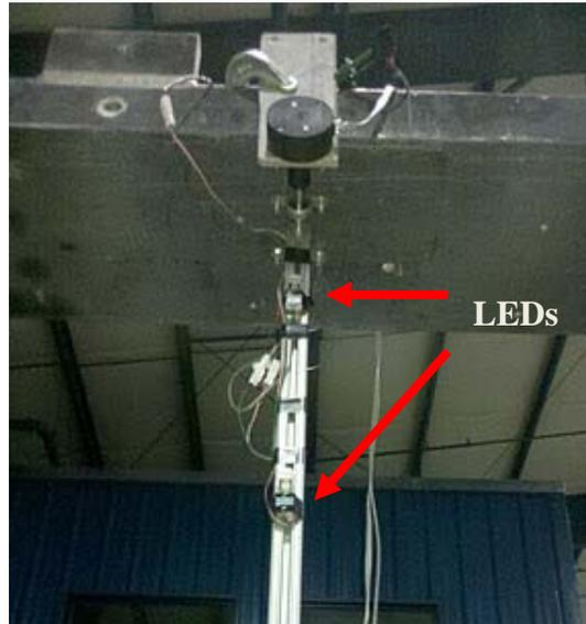
Figure 8: LEDs mounted to the pendulum.
