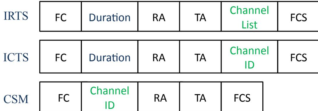
Figure 3.2: Structure of control frames used in *iMAC* protocol.
