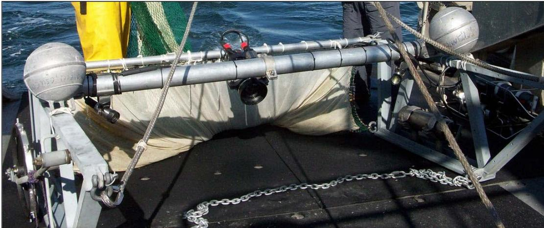
**Figure 3: Beam trawl used for capturing juvenile groundfish and epibenthic invertebrates.**
