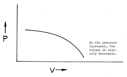
The top of the curve is normally flat. The top of the curve represents conditions which should be avoided.
