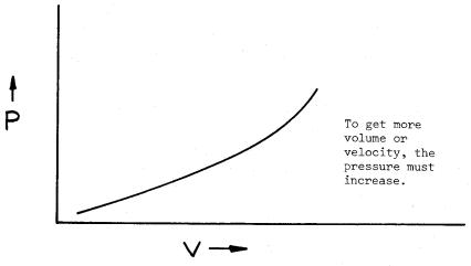
The curve will be parabolic having an exponent within the range of 1.5 to 2.
