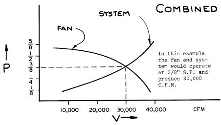
In the case of the D.T. kiln, the system resistance looks like the following curve.
