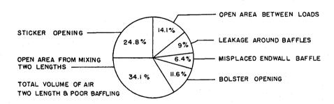
Note that only 24.8% of the air flow produced by the fans passes through the stickered openings.
