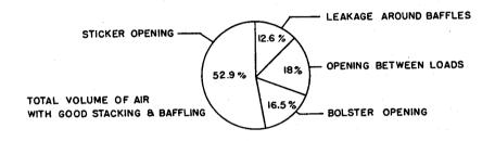
Note that because of the greater velocity through the larger openings, only 52% of the air flow produced by the fans passes through the sticker openings.
