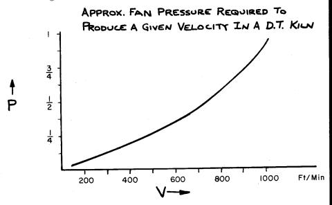
In this curve, the pressure is plotted against velocity. From this curve we can determine the static pressure the fan must operate under to provide the required air velocity.
