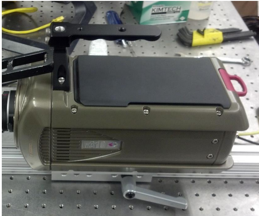
Figure 13: v310 high speed camera mounted on slide rail to allow adjustment of the position.
