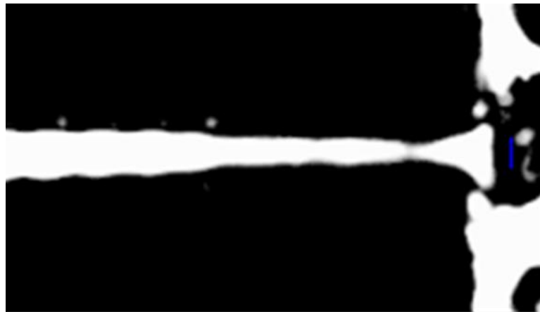
Figure 16: Line profile used to measure when a slug venting event occurred on the right side of the channel
