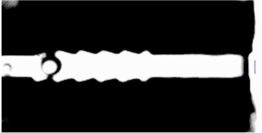
Figure 16: Line profile used to measure when a slug venting event occurred on the right side of the channel
