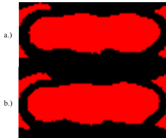
Figure 18: Sequential perturbation of color threshold parameters for binarizing the image for processing. a.) All parameters set at 10. b.) All parameters set at 250. This represents the start (a.) and end (b.) of the sequential perturbation analysis
