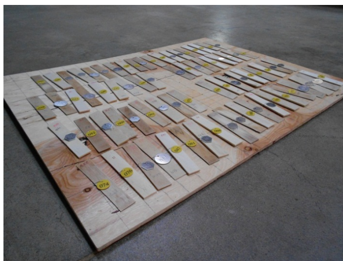
Figure 4 - Formosan termite test array with VTC and non-VTC processed veneers attached
