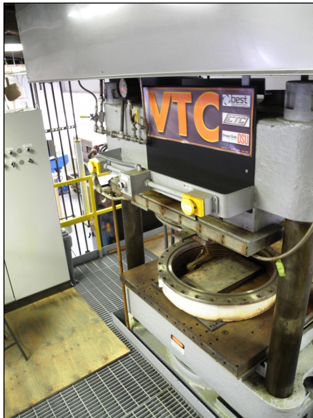
Figure 1 - VTC densification chamber at the Oregon State University Green Building Materials Laboratory
