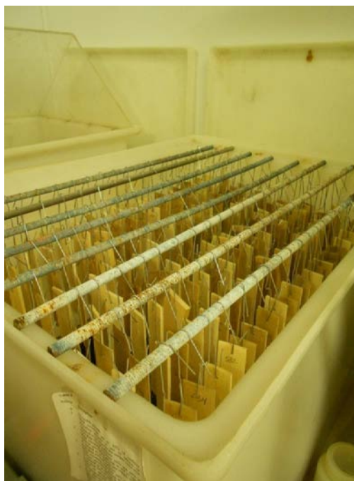
Figure 6 - Hybrid poplar veneer specimens placement within a mold box
