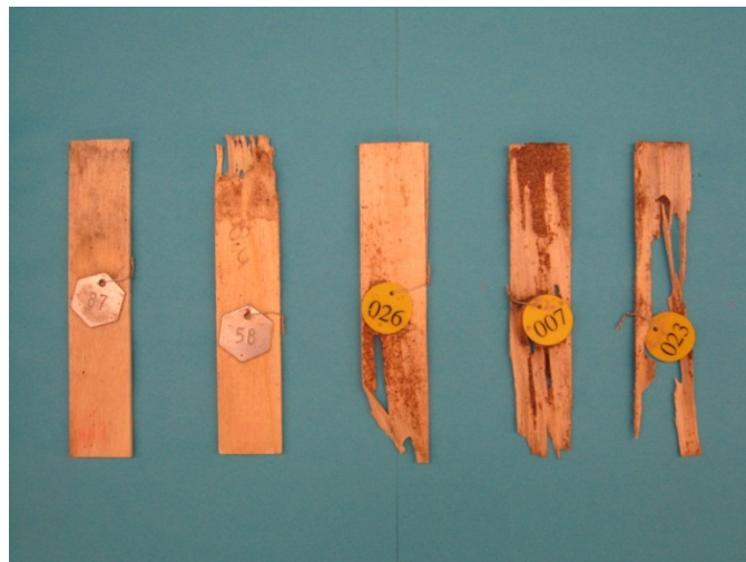
Figure 17 - Hybrid poplar veneer specimens with five degrees of termite attack rating of 10,9,7,4,and 0 (left to right)
