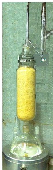
Figure 3 - Steam distillation device used to collect western juniper oil
