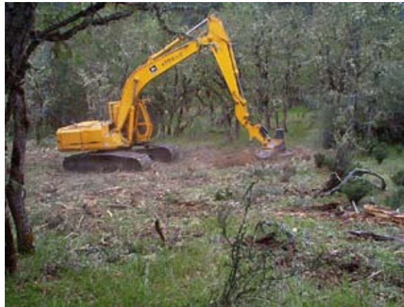
Figure 1. Slashbuster equipped with rotating head. Photo: Ed Reilly, Bureau of Land Management.
