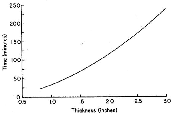
Figure 5. Effect of thickness on the time required to press dry loblolly pine 2 by 4's from 120 to 15 percent moisture content at 350° F platen temperature. (ML88 5621)
