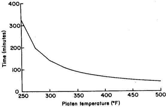
Figure 4. Effect of platen temperature on the time required to press dry loblolly pine 2 by 4's from 120 to 15 percent moisture content. (ML88 5620)
