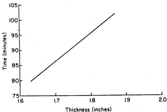
Figure 6. Effect of thickness variation around a target thickness on the time required to press dry loblolly pine 2 by 4's from 120 to 15 percent moisture content at 350° F platen temperature. (ML88 5622)
