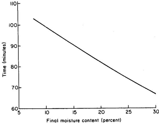
Figure 3. Effect of final moisture content on the time required to press dry loblolly pine 2 by 4's from 120 percent initial moisture content at 350° F platen temperature. (ML88 5619)
