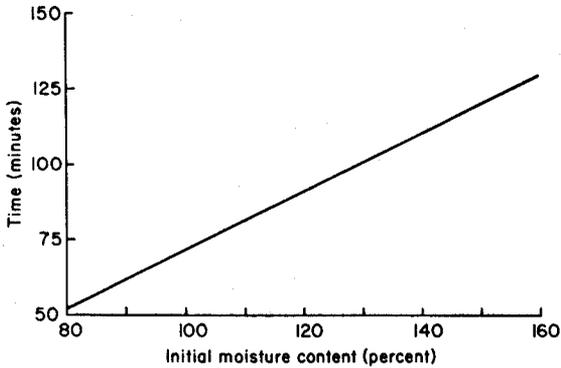
Figure 1. Effect of initial moisture content on the time required to press dry loblolly pine 2 by 4's to 15 percent moisture content at 350° F platen temperature. (ML88 5617)
