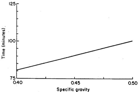
Figure 2. Effect of specific gravity on the time required to press dry loblolly pine 2 by 4's to 15 percent moisture content at 350° F platen temperature. (ML88 5618)
