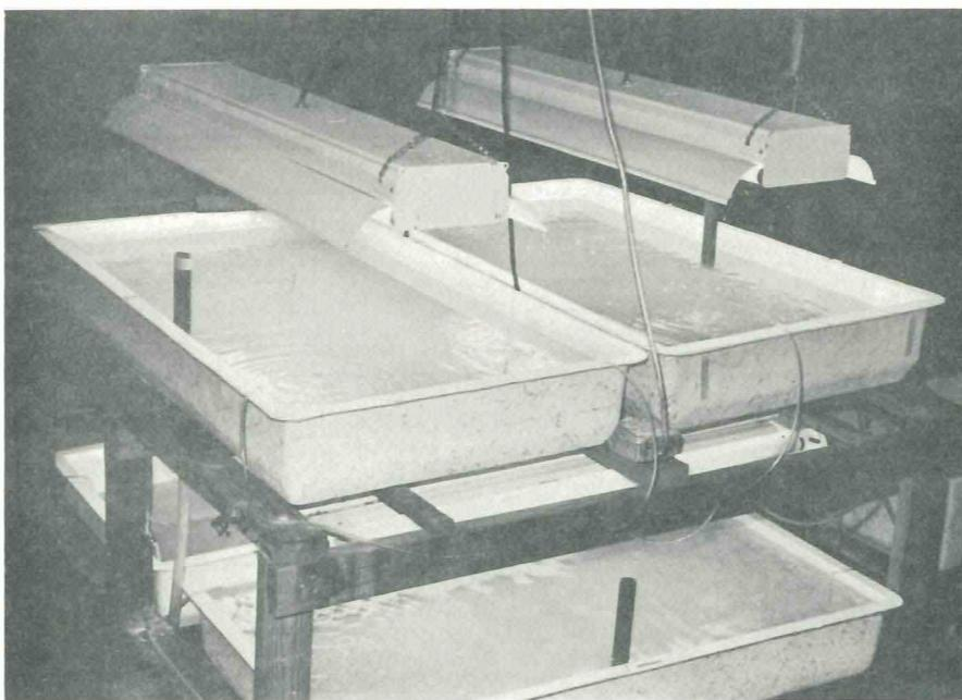
Figure 4. Fiberglass tanks for mass culture of algae
