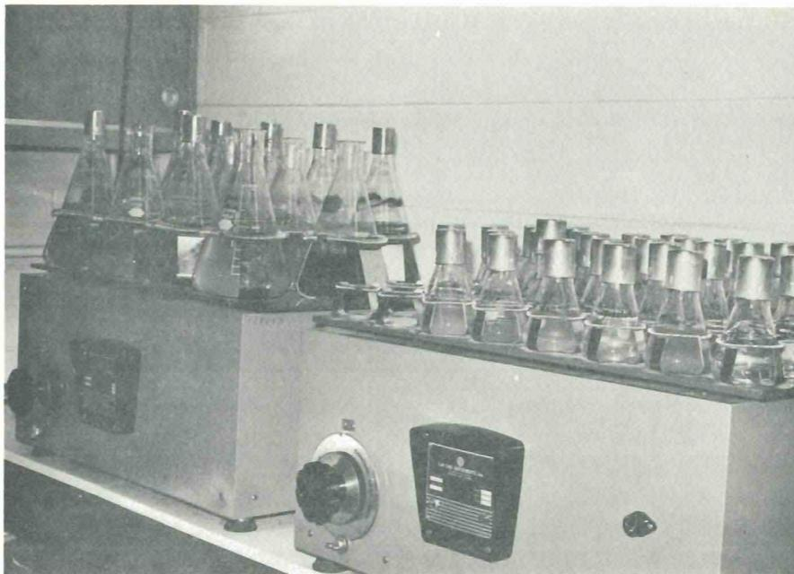
Figure 3. Unialgal cultures maintained in flasks on orbital shakers
