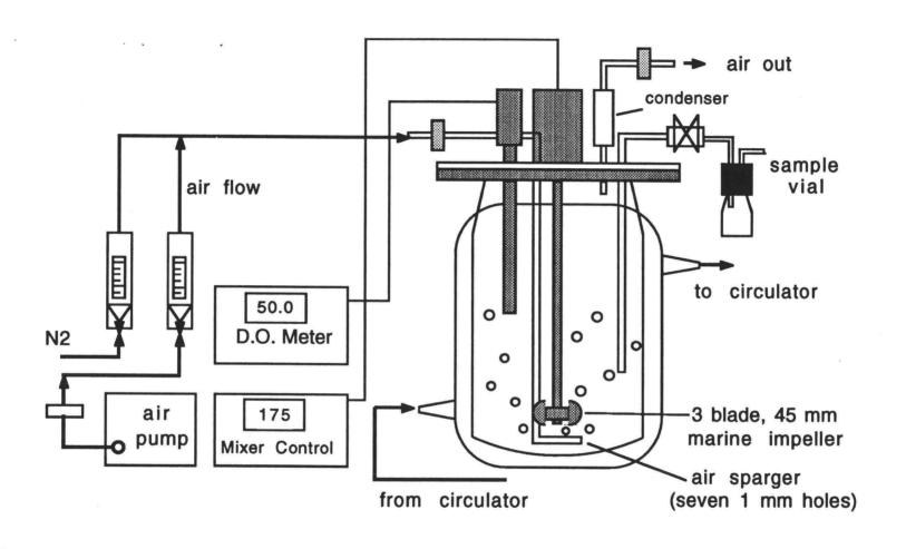
Fig. 1. Three liter Applikon Stirred-Tank Bioreactor
