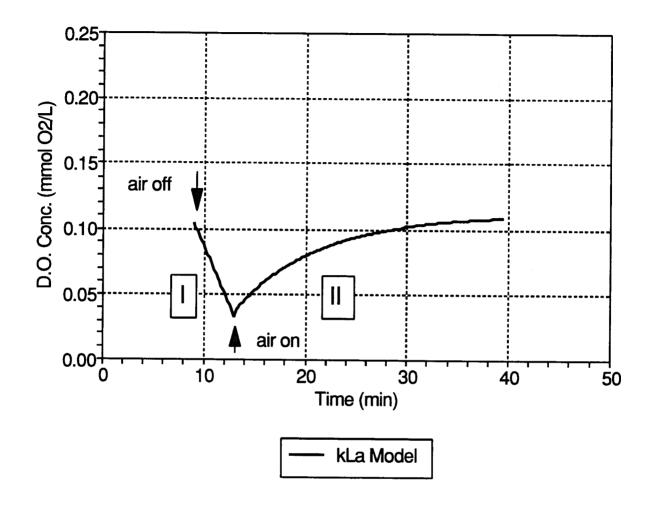
Figure 3b. Estimation of Qo and culture k<sub>L</sub>a by the dynamic method Cultivation conditions: impeller speed, 175 rpm; aeration rate, 0.43 vvm; cultivation hour, 91 hr; total cell density, 5.4 g DCW/L.
