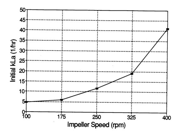
Figure 2. Initial k<sub>L</sub>a vs. mixing speed at 0.43 vvm aeration rate.
