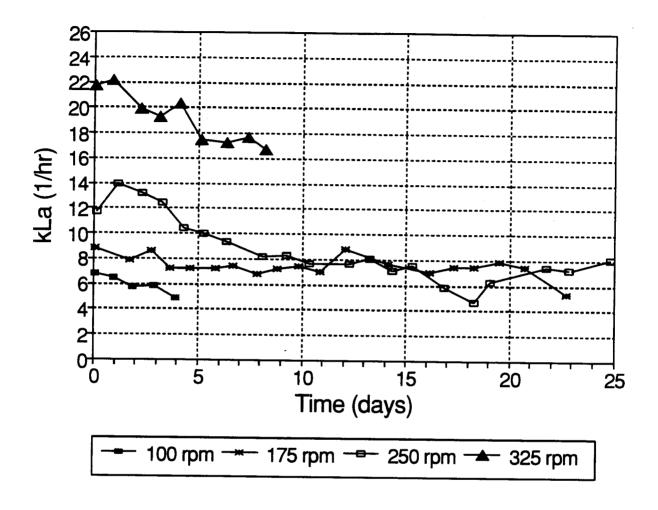
Figure 24. Culture k<sub>L</sub>a at impeller speeds of 100 to 325 rpm.
