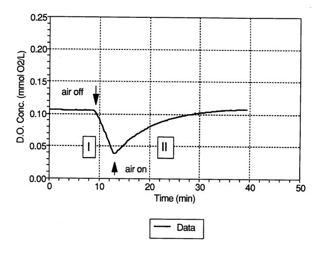
Figure 3a. Estimation of Qo and culture  $k_L a$  by the dynamic method Cultivation conditions: impeller speed, 175 rpm; aeration rate, 0.43 vvm; cultivation hour, 91 hr; total cell density, 5.4 g DCW/L.
