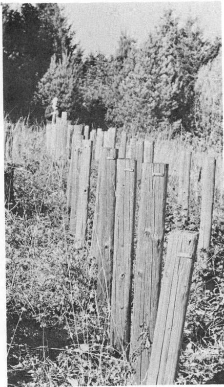
Damp-wood termites swarm during late summer and early fall. At time of annual inspection in early October, discarded wings of reproductives have been found at bases of many posts. Entry holes have been made at or below ground line. In only a few instances have termites been the primary cause of failure.
