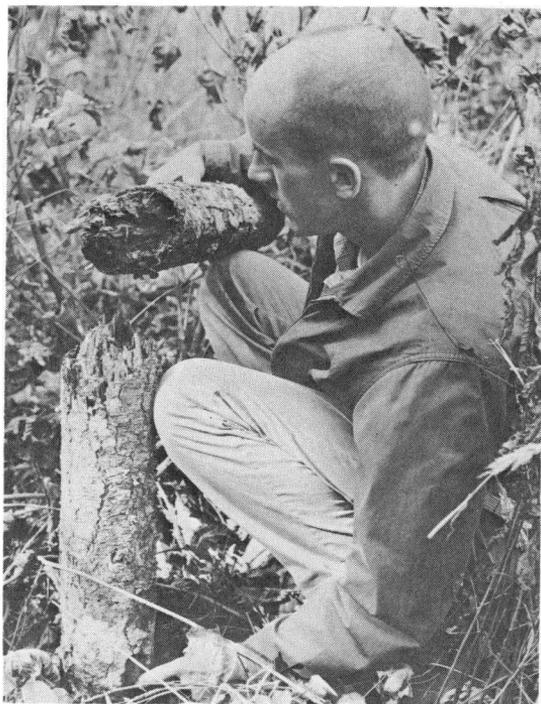
Figure 5. Tops of Douglas fir posts were not protected adequately when chemicals were placed in holes drilled near the ground line of undried, unpeeled posts.
