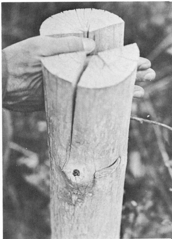
Figure 7. After 12 years in service, Oregon maple that was soaked in 5 per cent pentachlorophenol-diesel oil had 92 per cent of posts remaining. Many tops of these posts were split.
