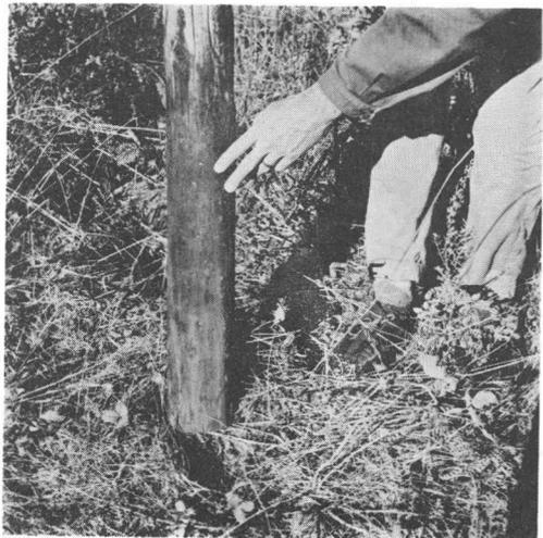
Figure 4. After 31 years in service, Douglas fir posts were in good condition because of pressure treatment with coal-tar creosote.
