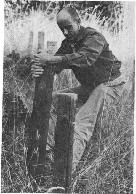
Figure 2. During annual inspection, each post received a moderate pull at the top to test for failure.
