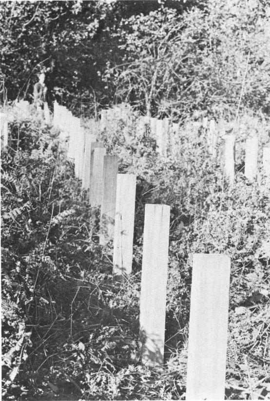
Figure 6. Posts of West Coast hemlock that were pressure-treated with Chemonite and Wolman salts had 96 per cent remaining in service after 23 years.
