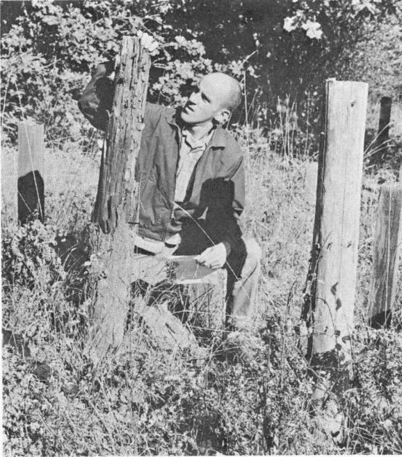
Figure 3. Undried Douglas fir posts received an end-diffusion treatment with Chemo-nite by the tire-tube method. Service life was increased, but where bark remained on posts, most tops contained decay.
