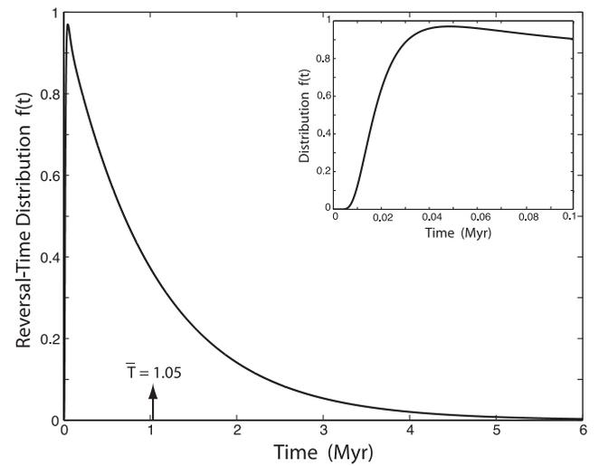
**Figure 8.** Reversal time distribution,  $f(t)$ , computed from a numerical solution of the Fokker–Planck equation with an initial condition  $x(0) = 5.3 \times 10^{22} \text{ A m}^2$ . After a short transient (inset) the probability distribution decreases exponentially with  $t$ .
