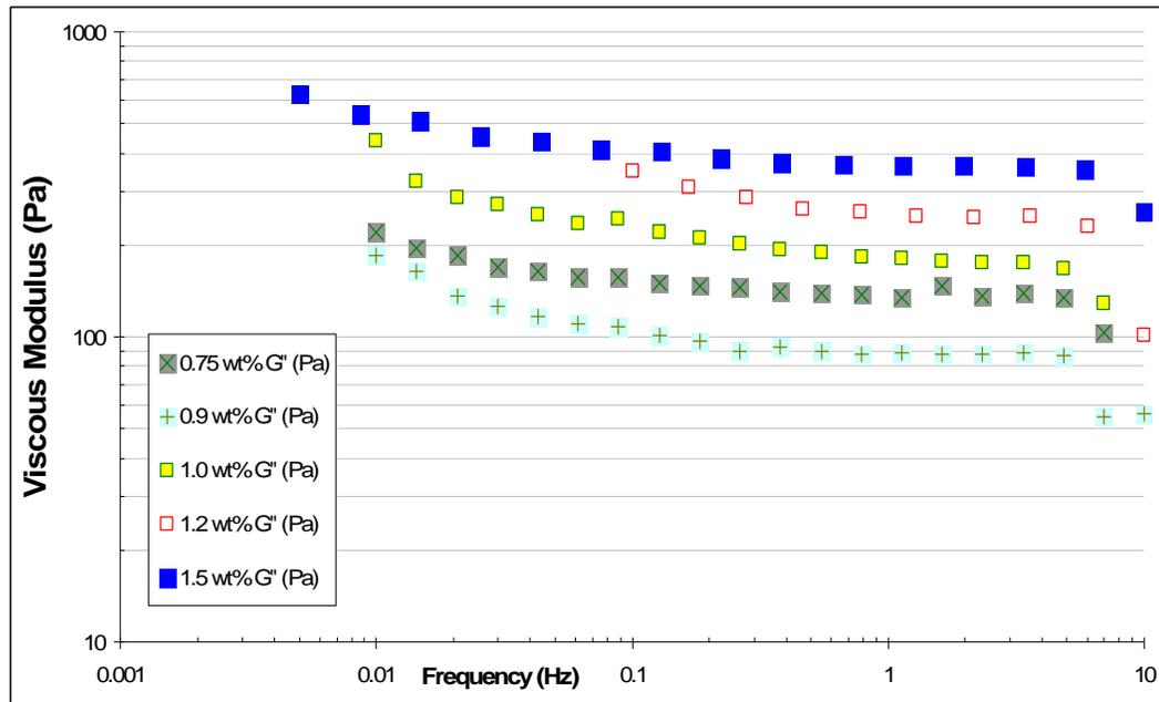
Figure 16: Frequency sweep performed at  $\gamma = 0.05$  for different weight percents of agarose gel showing Viscous Modulus values.
