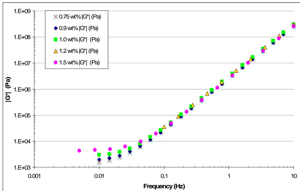
Figure 13: Frequency sweep performed at  $\gamma = 0.05$  for different weight percents of agarose gel showing  $|G^*|$  – Complex Modulus values.
