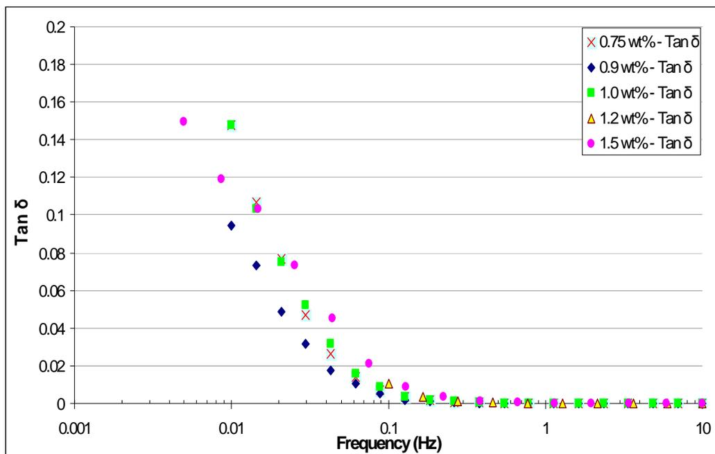
Figure 134: Frequency sweep performed at  $\gamma = 0.05$  for different weight percents of agarose gel showing  $\tan \delta$  values.
