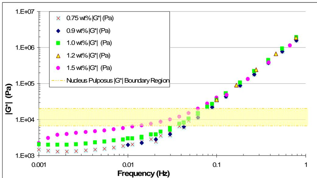
Figure 28: Frequency sweep performed at  $\gamma = 0.05$  for different weight percents of agarose gel showing  $|G^*|$  – Complex Modulus values and a boundary region of complex moduli from the Nucleus Pulposus under the same loading mode.
