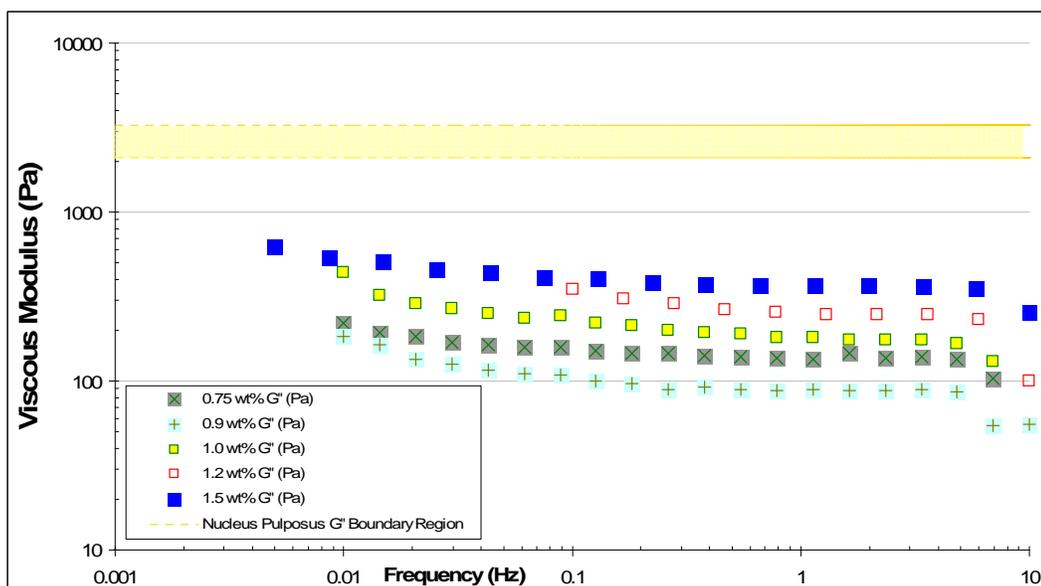
Figure 27: Frequency sweep performed at  $\gamma = 0.05$  for different weight percents of agarose gel showing  $G''$  values and a boundary region of viscous moduli from the Nucleus Pulposus under the same loading mode.
