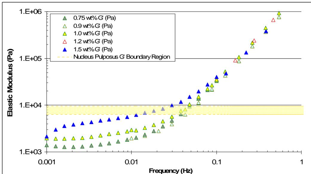
Figure 26: Frequency sweep performed at  $\gamma = 0.05$  for different weight percents of agarose gel showing  $G'$  values and a boundary region of elastic moduli from the Nucleus Pulposus under the same loading mode.
