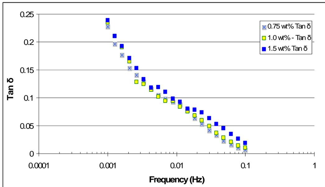
Figure 18: Small frequencies sweep performed at  $\gamma = 0.05$  for different weight percents of agarose gel showing  $\tan \delta$  values.
