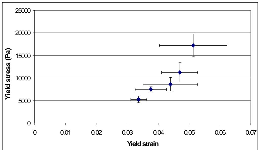
Figure 24: Yield stress versus yield strain at each weight percent of agarose gel.
