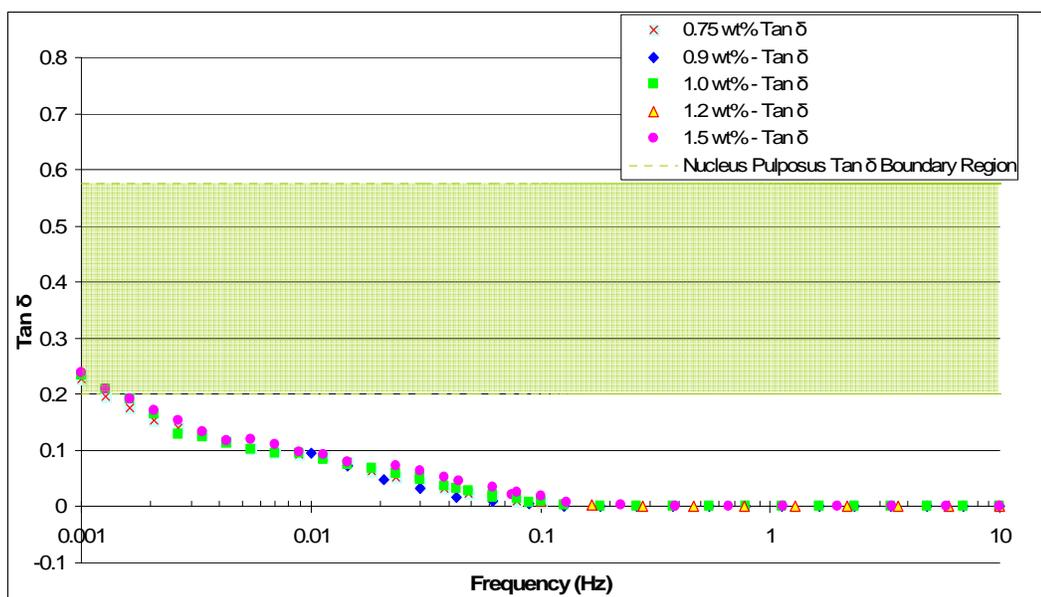
Figure 29: Frequency sweep performed at  $\gamma = 0.05$  for different weight percents of agarose gel showing  $\tan \delta$  values and a boundary region of  $\tan \delta$  from the Nucleus Pulposus under the same loading mode.
