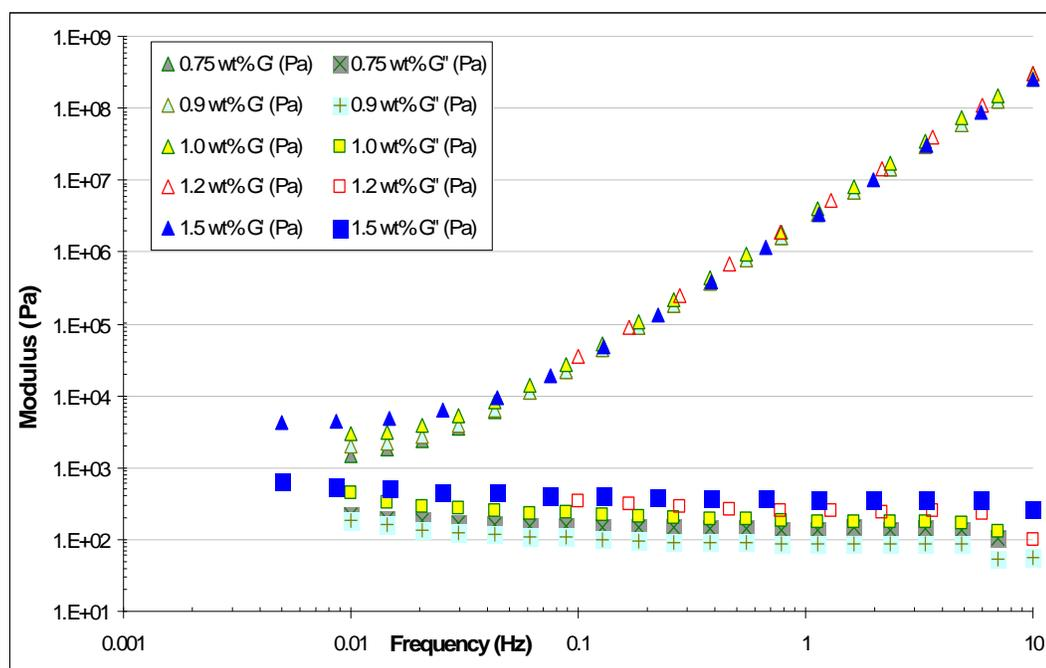
Figure 15: Frequency sweep performed at  $\gamma = 0.05$  for different weight percents of agarose gel showing Elastic and Viscous Modulus values.
