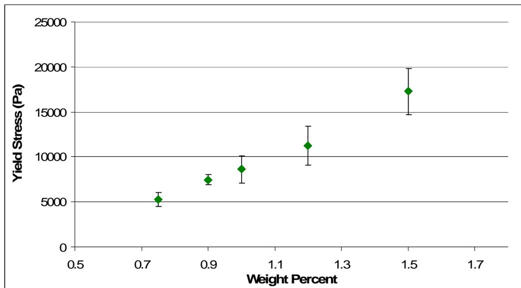
Figure 22: The stress value for each gel when the material yielded (extrusion from the cavity).
