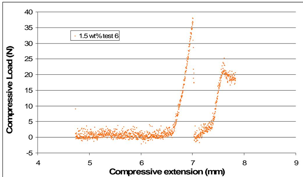
Figure 20: Typical raw compressive data plot for a 1.5 weight percent agarose gel
