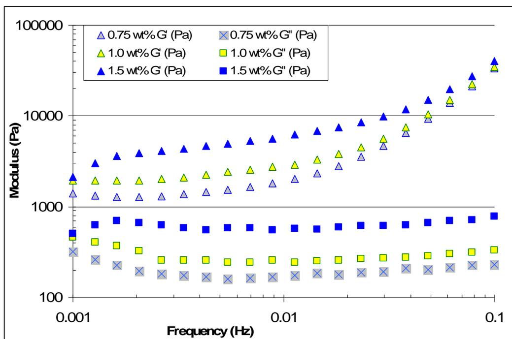
Figure 17: Small frequencies sweep performed at  $\gamma = 0.05$  for different weight percents of agarose gel showing Elastic and Viscous Modulus values.
