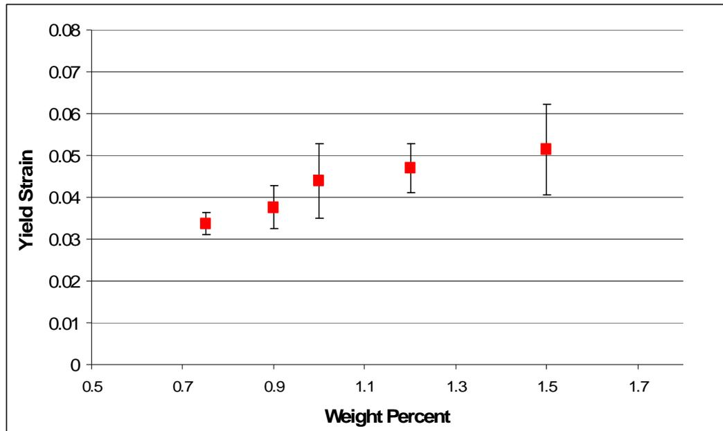
Figure 23: The strain value for each gel when the material yielded (extrusion from the cavity).
