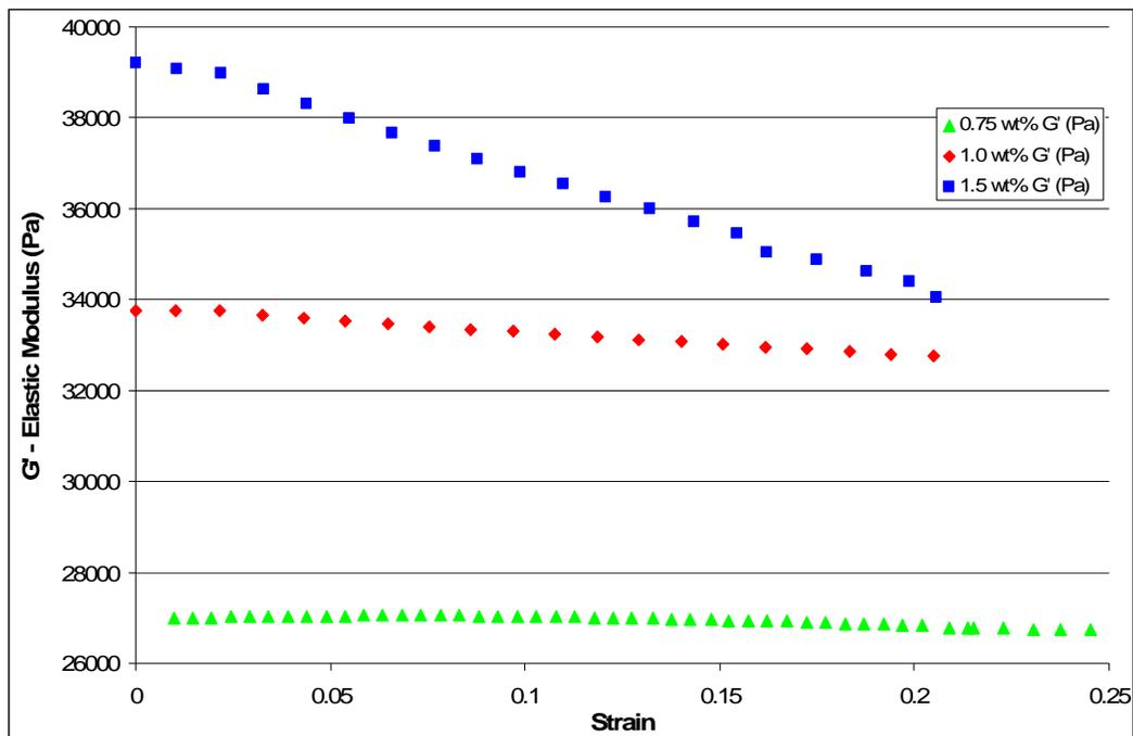
Figure 12: Strain amplitude sweep performed at 0.1 Hz for different weight percents of agarose gel showing  $G'$  – Elastic Modulus values.
