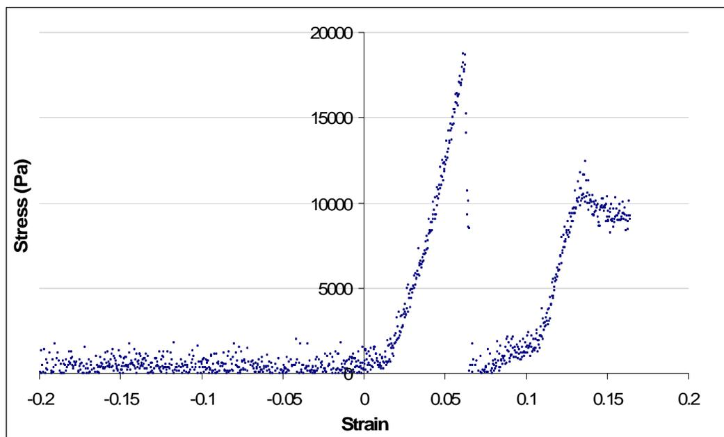
Figure 21: Typical stress - strain plot for a 1.5 weight percent agarose gel.
