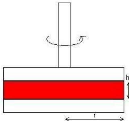
Figure 10: Parallel plate geometry.
