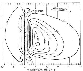
Percentage of normal wind velocity near a windbreak having an average density of 50 percent. (Redrawn from Bates, 1944.)
