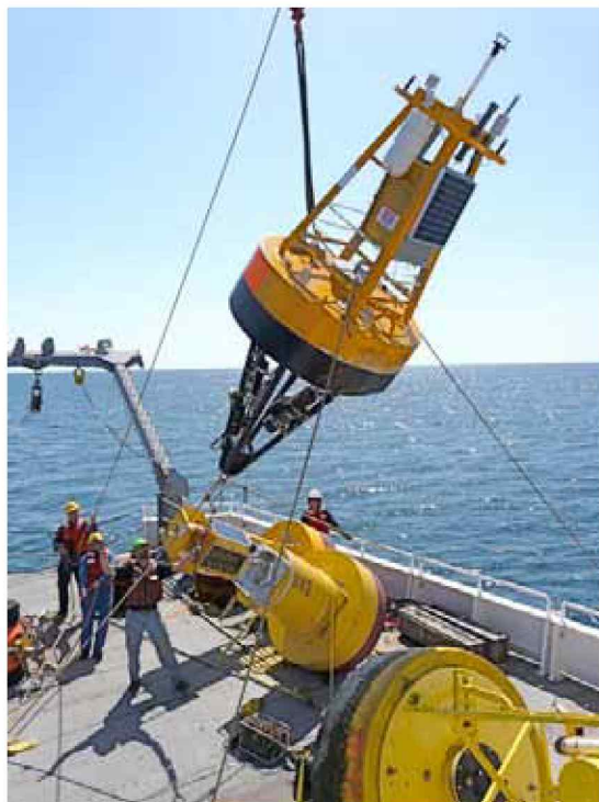
The Multi-Function Node is deployed off of Yaquina Head in support of the Ocean Observation Initiative
