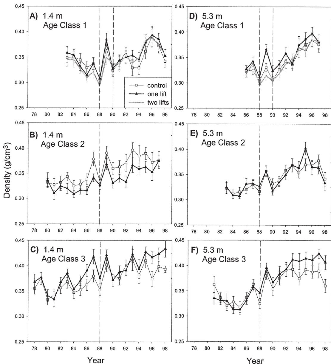
FIG. 2. Radial patterns of wood density by pruning treatment at breast height (1.37 m) and at the upper height (5.3 m) for each of the three age classes (mean  $\pm$  s.e.,  $n=12$  trees for each data point). The dashed lines show when trees were pruned.
