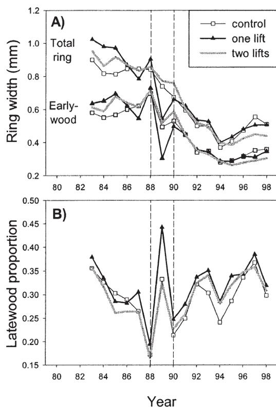
FIG. 1. Radial patterns of growth-ring width by pruning treatment at breast height (1.37 m) for age class 1 (mean  $\pm$  s.e.,  $n=12$  trees for each data point). A) Total growth-ring width and earlywood growth ring width. B) Latewood proportion. The dashed lines show when trees were pruned.
