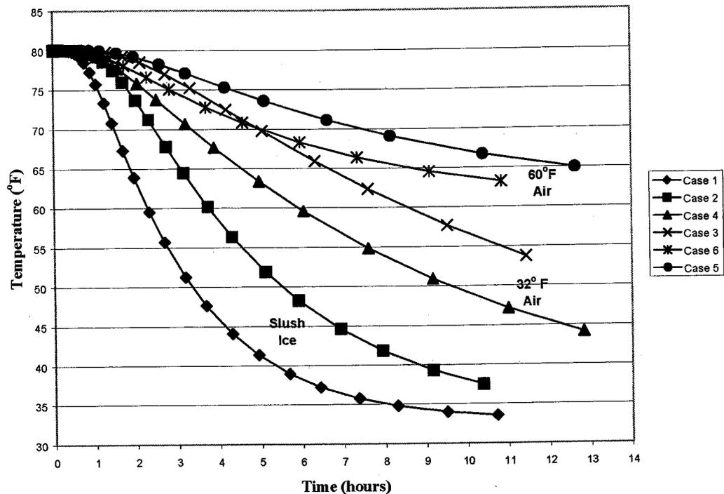
**Figure 2.** Simulation showing effects of fish size and ambient conditions on chill rate.
