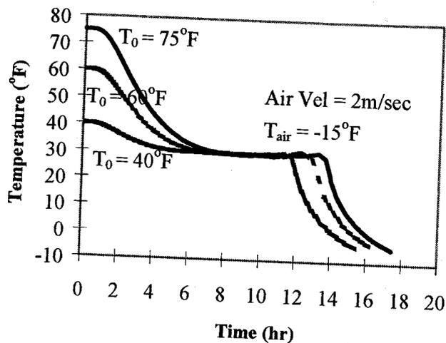
**Figure 9.** Effects of pre-chilling on blast-freezing of a large (24-lb) fish.
