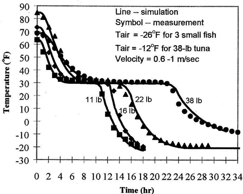
Figure 4. Blast freezing of four sizes of fish.
