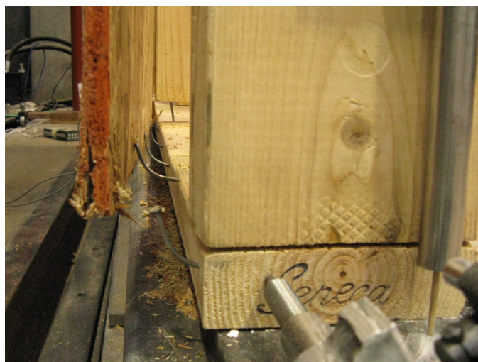
Fig. 8. Two failure modes were observed: pullout and bending of sheathing nails (occasional pull-through) and separation of framing members
