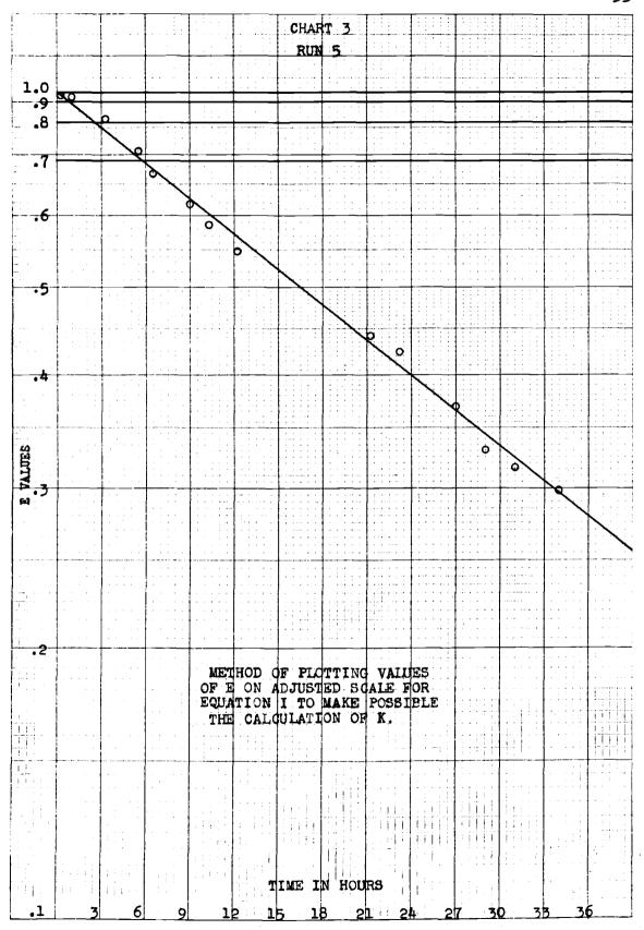
Using run number five as an example, from the table on page 31,  $K\Theta/R^2$  is .25 when E is .450. From the chart of run number five, page 35, it will be noted that the time is 20.75 hours at this E value. The thickness is one inch. Therefore to solve for E the equation becomes,
