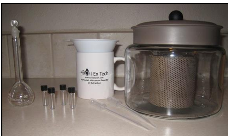
Figure 2.3.6: Essential Oil Extraction Device from OilExTech™ LCC Plant material is loaded into the glass container around the condensate cup. An ice core attached to the lid condenses the steam and oil vapors which drip down into the condensate cup. A typical extraction takes around 10 minutes from start to finish. 28
