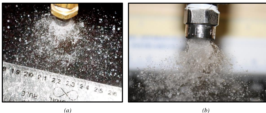
Figure 5.2.2: Lechler 460.528 Full Cone Nozzle Spray Detail
