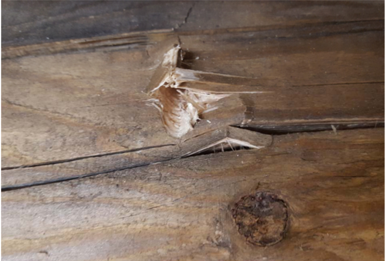
Figure 5-8: Compression failure marked by buckling of wood fibers around the hole.
