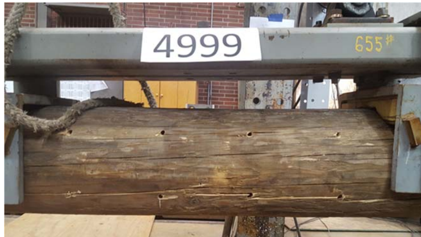
Figure 3-4. Example of a hole pattern used to through bore Douglas-fir poles. Holes with an “x” were not drilled.
