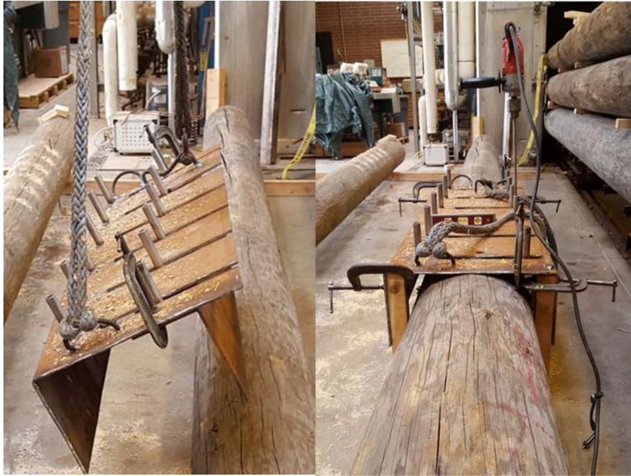
Figure 3-2 and 3-3. Photos of the drilling apparatus created for drilling holes at a constant edge distance. The plate can slide in and out to fit any size. Blocks cut to 1 and 2 inches are placed in the interior edges to drill at different edge distances. Holes are drilled downward through the pipes.
