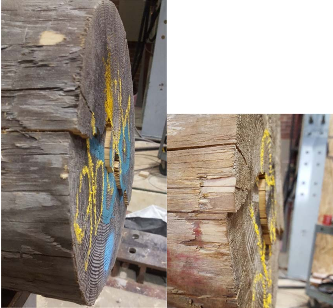
Figure 5-7: Two end shear failure at the pole end, marked by separation of the areas above and below the center of the pole.
