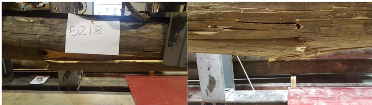
Figure 5-6: Tensile failures caused by failure at a knot and rupture of fibers.
