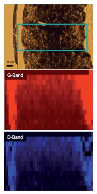
Figure 2. The top image is the sample to be analyzed; the left hand side is the dorsal surface of the sectioned *Daphnia magna* the blue square is the area analyzed by Raman Spectroscopy. The G-band and D-band signals are strong in the gut and absent at the edges indicating a high concentration of ingested OH-SWCNTs within the gut but no detectable signal in the tissues.
